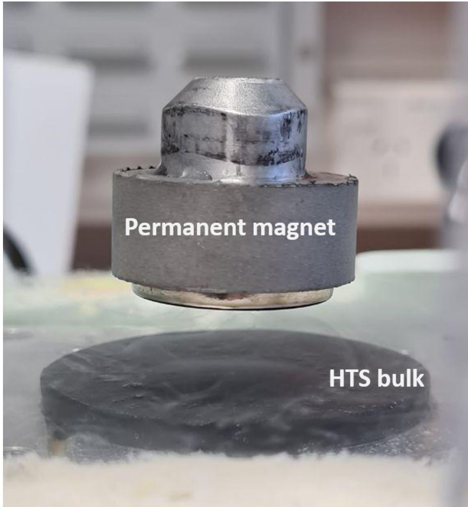
Figure 1.1: Photo of a NdFeB PM levitated above an YBCO bulk submerged in liquid nitrogen used in this thesis work.
