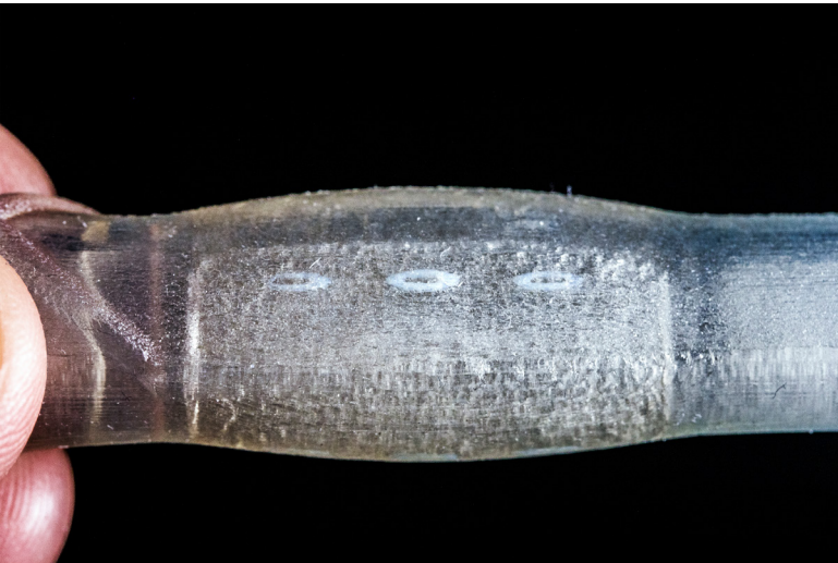
Figure 88. Gills on the pneumatic valve to release air, in an attempt to prevent the material from splitting due to over inflation.
