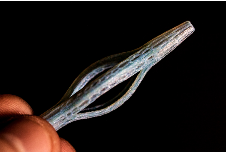
Figure 100. An investigation into Vero Voronoi forms to increase the strength of the bands.
