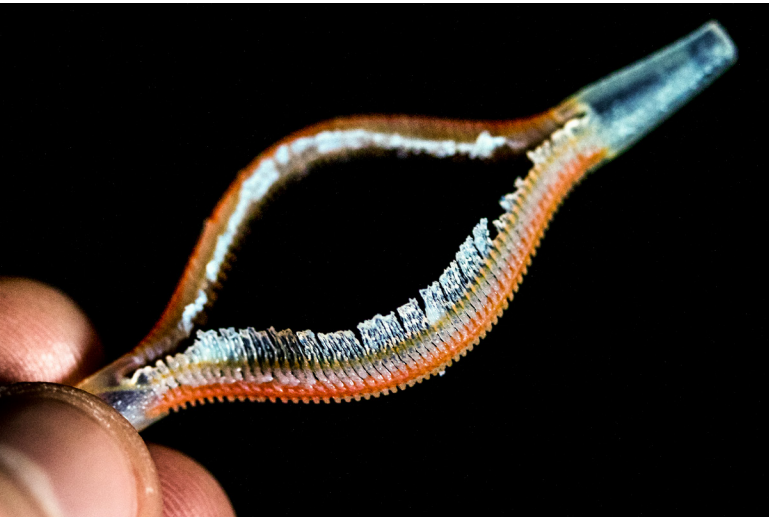
Figure 104. Thin strands of support started printing within the fins when the size of the bands increased. The support would not dissolve in the DT3 cleaning bath.
