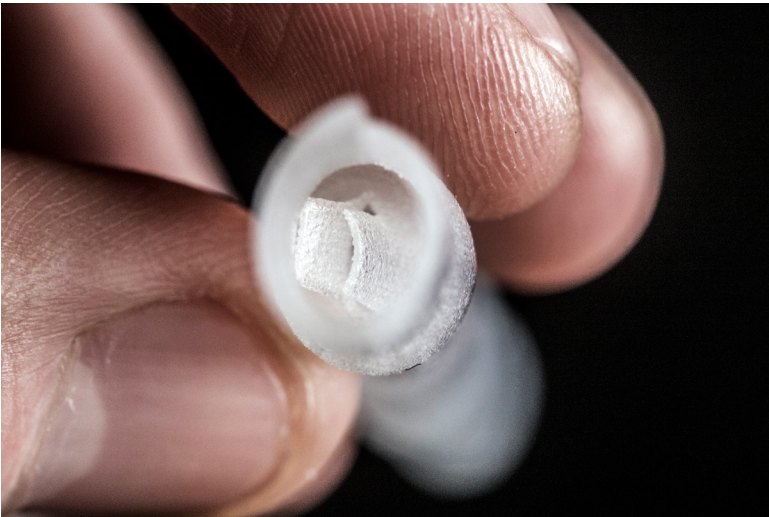
Figure 84. Exploring valve leaflets at a smaller scale to assess the J750's capabilities, the tubes inside diameter is 5mm.
