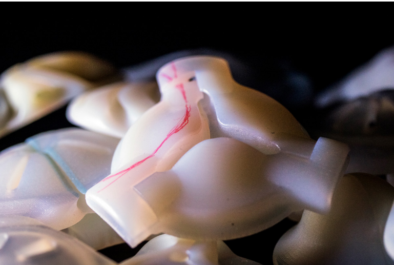
Figure 70. Sketching on prototypes signified changes. The red lines indicate the excess material to remove on the next iteration.
