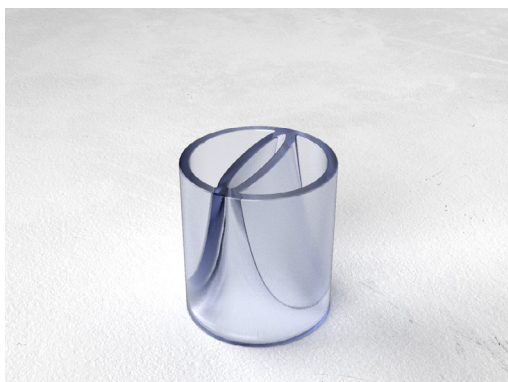
1. Bicuspid leaflets merged with wall, failed to open.
