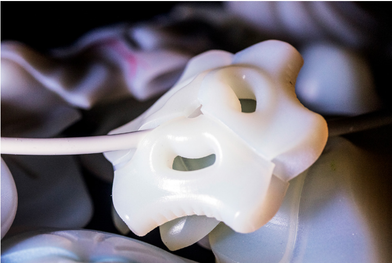
Figure 69. Drains popping out of the slit was a frequent issue.
