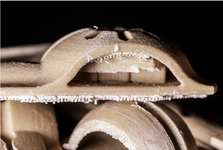
Figure 65. Support material proved to be an issue with FDM printing.
