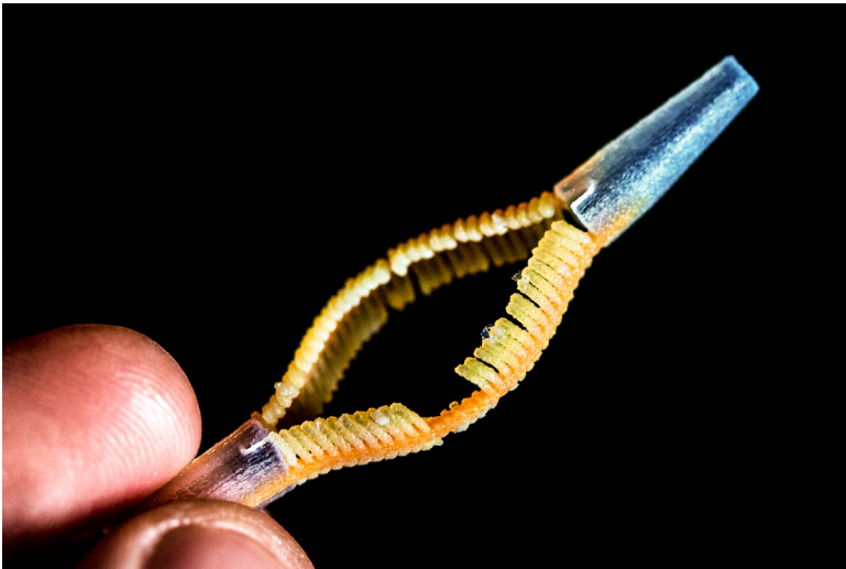
Figure 101. Thin strands of Vero were printed within the fins to provide more strength; however, some fins still broke off during cleaning.
