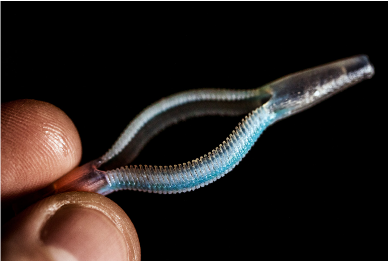
Figure 102. Printing a thin strand of Vero piercing through all the fins provides enough strength to survive cleaning.
