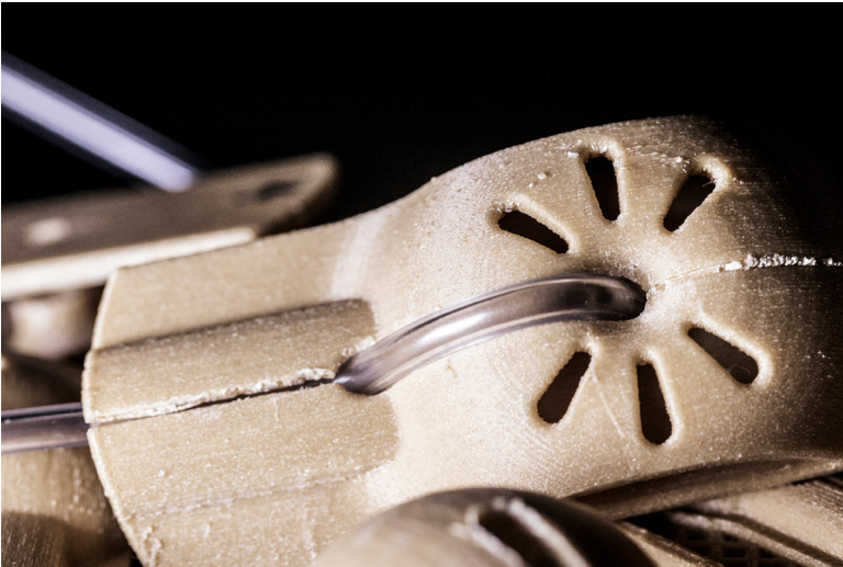
Figure 64. Early low fidelity prototypes of the skin fixation device were generated with FDM 3D printing (Fused-Deposition-Modelling).
