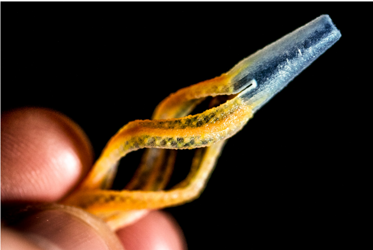
Figure 105. An investigation into internal lattice structures within the bands of a Helix drain.
