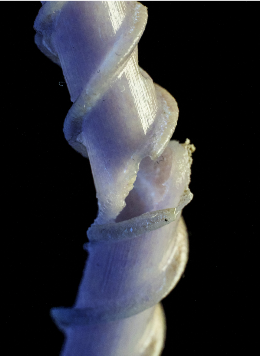
Figure 144. Tight External Spiral irrigation drain splitting during the removal of the internal stent.
