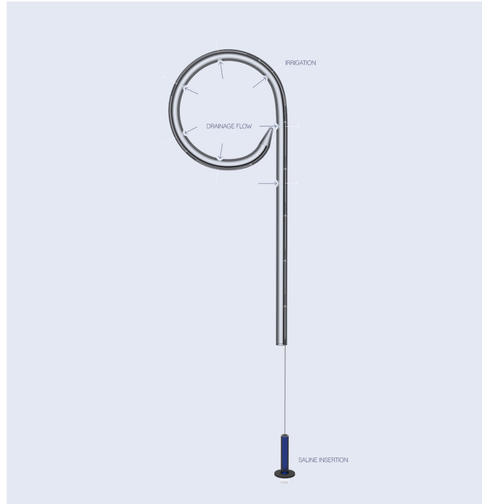
Figure 96. Double lumen irrigation renders and flow diagram, to understand the most efficient configurations for irrigation and drainage.
