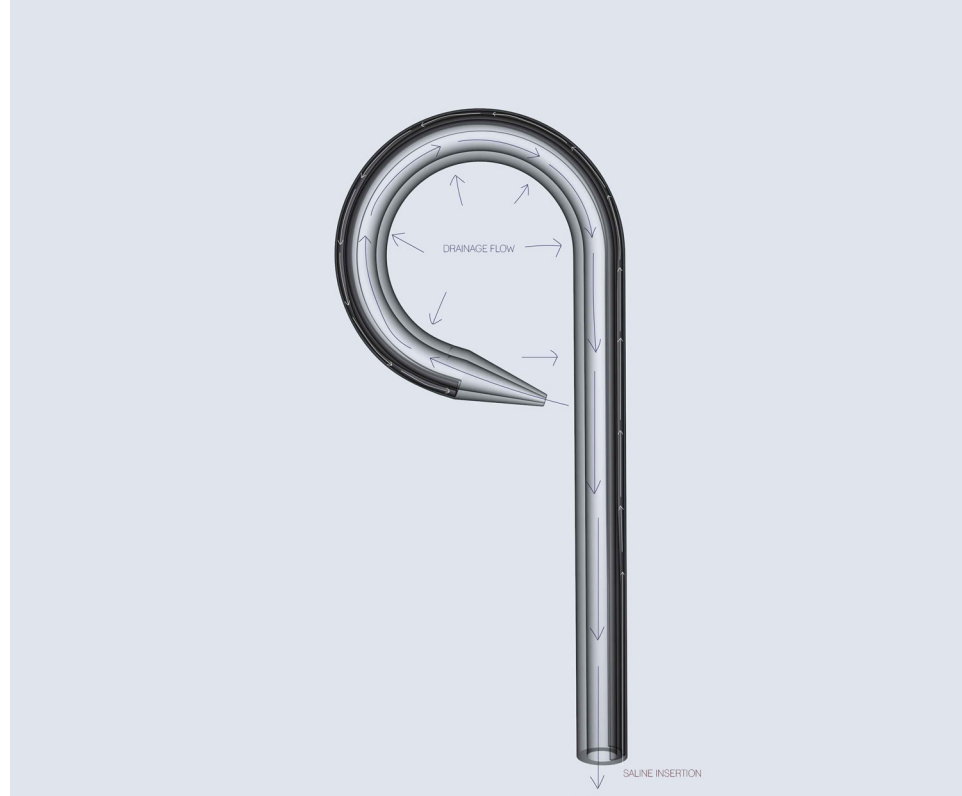
Figure 78. Developed blow-up Pigtail renders and flow rate diagram, creating an understanding of how the cavity within the walls, creates a breathing effect through fluid or air and material manipulation.
