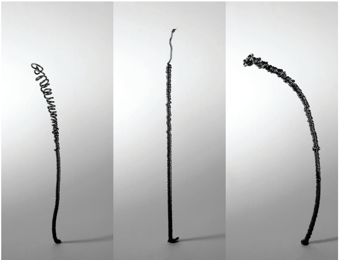
Figure 34. Helical test failure modes
