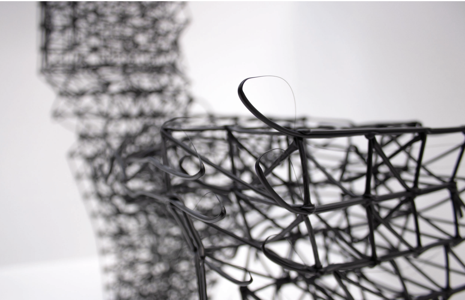
Figure 55. Rapid movement related print issues.
