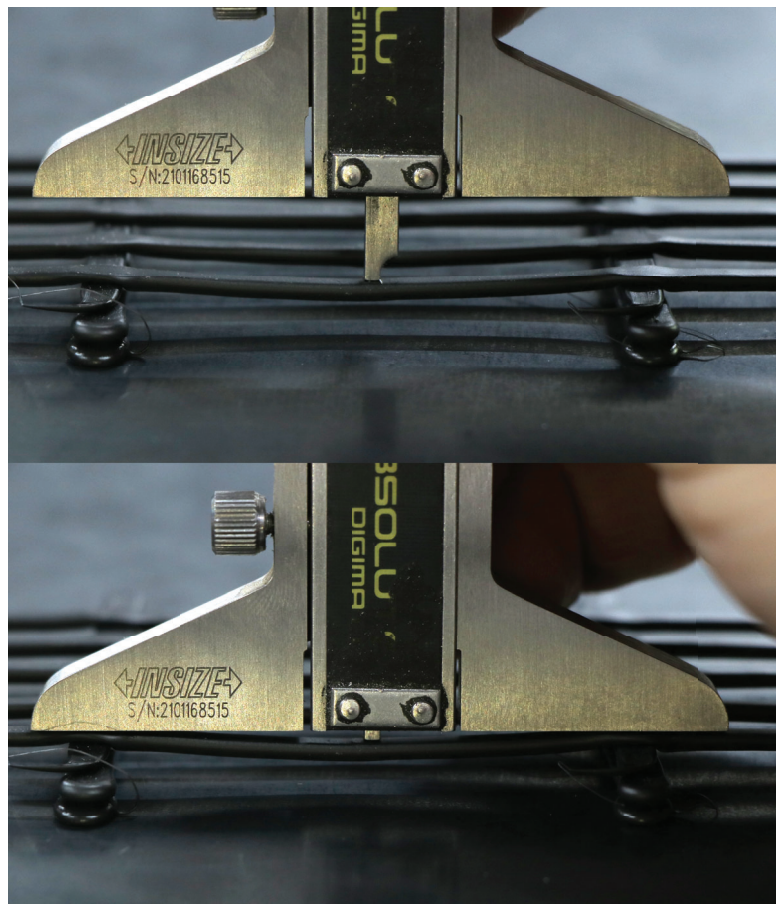
Figure 29. Digital calipers were used to measure how much each bridging element had bowed.
