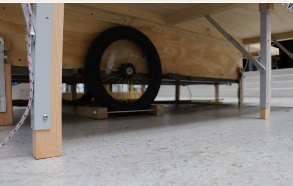
Fig 119. Chocks stabilise the cart and the legs are adjusted with screws. ↓
