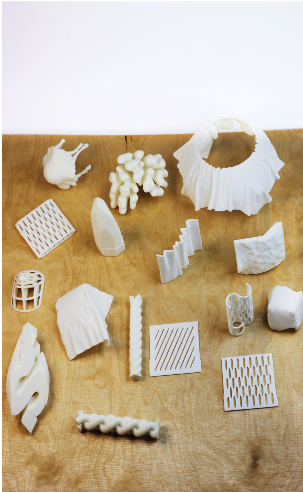
Figure 3.1 - Collection One, all made using ABS FDM printing, showcasing various possibilities for exploring VTIs.
