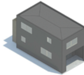
Figure 165: Small design at single garage size. Shown on a concrete subfloor so that it can function as a garage at some time in its life. The design can easily be altered for a timber subfloor if its unlikely it will used as a garage
