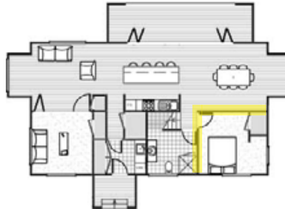
Figure 160: Large Version Ground Floor Plan. The yellow shaded walls indicate soundproofing. Note sound proofing will also be provided in any adjacent floors/ceiling/walls to other spaces on the first floor.
