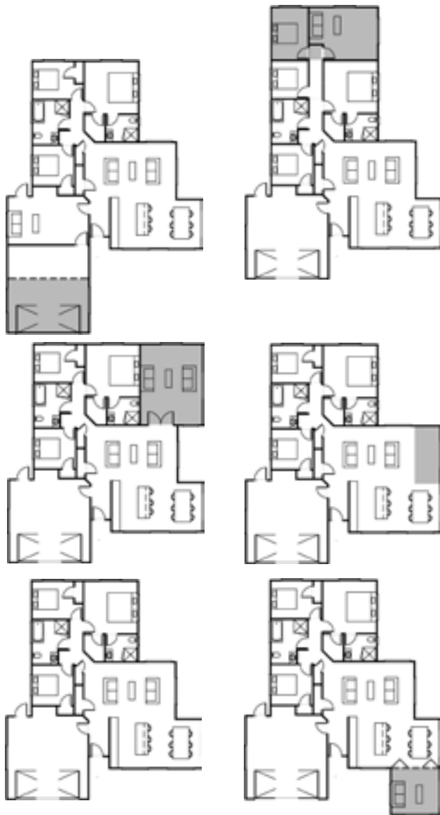
Figure 55: Left: Grey shaded area indicates different floor plan options for additions to Punto through lean-to, and adding onto the hip roof. Adding a lean-to is trailed on Punto though the low stud height renders it impracticable. The only option then is to construct the new extension over the existing hip roof as shown. The extensions have been shown as a hipped roof to keep with existing style though a gable would be more suitable if future additions were possible.
