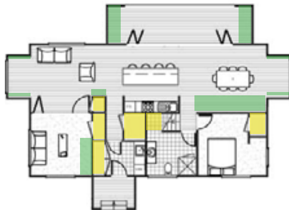
Figure 138: Large Version: Ground Floor Plan. The yellow shading indicates built in cupboards. The green shading indicates possible future locations of storage either built in or free standing.
