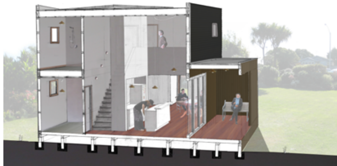
Figure 141: Section through the double height space of the large design. A floor has been added into part of the double height space at a later date.
