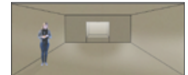
Light enters indirectly through a hidden skylight or side light
