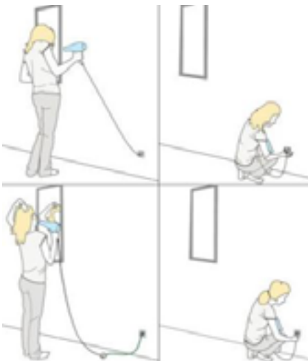
Figure 46: Extension cord built into the wall.
