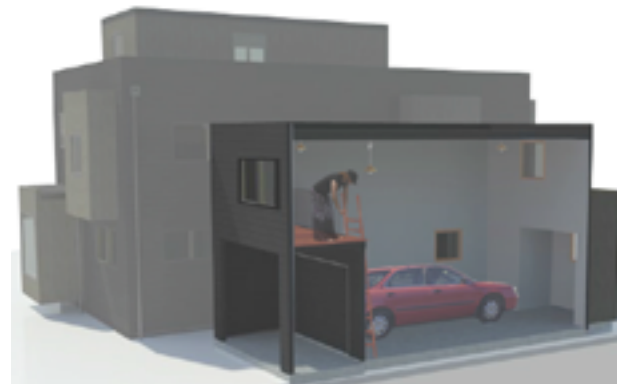
Figure 168: Sectional perspective and plan. In the front of the add on, an overhang provides a covered area which can be particularly useful for a workshop where maximum natural light or ventilation may be required with cover from rain. The overhang also provides a pleasant space for outdoor living if the garage space was adapted into a habitable space.
