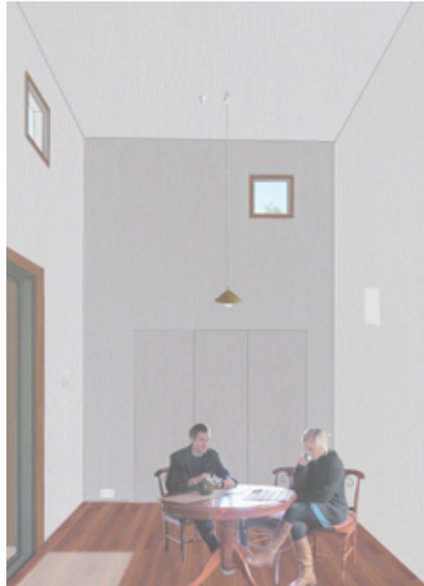
Figure 149: The link could be shut off from the main space with large bi-fold doors. The bi-fold doors could have an STC rating for acoustic privacy.
