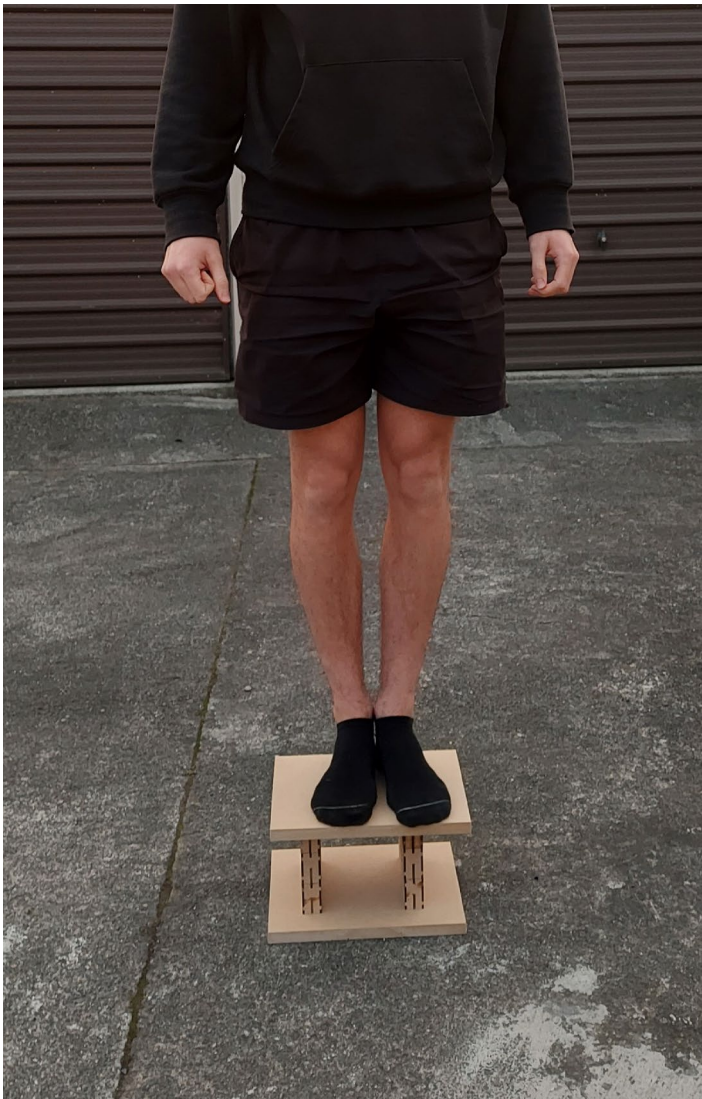
Figure 72. Vertical strength test using authors weight (a).
