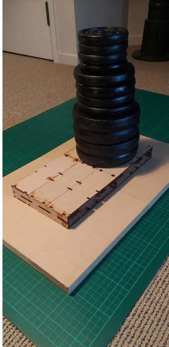
Figure 68 & 69. Testing various weights on a scale model of ClickBlock (a).
