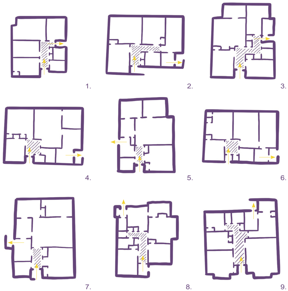
Fig. 9-17. State house floor plans showing circulation
