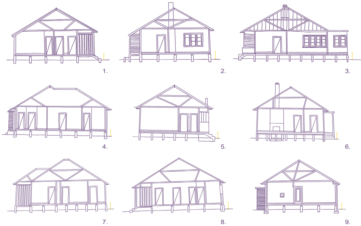
Fig. 36-44. State house sections showing floor height
