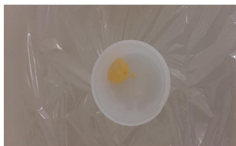
Figure 3.3a. Photo of first stage dried down coral standard material, including distinct orange colour and bubbly gelatinous form. The orange colour was maintained in solution through subsequent digestion procedures.
