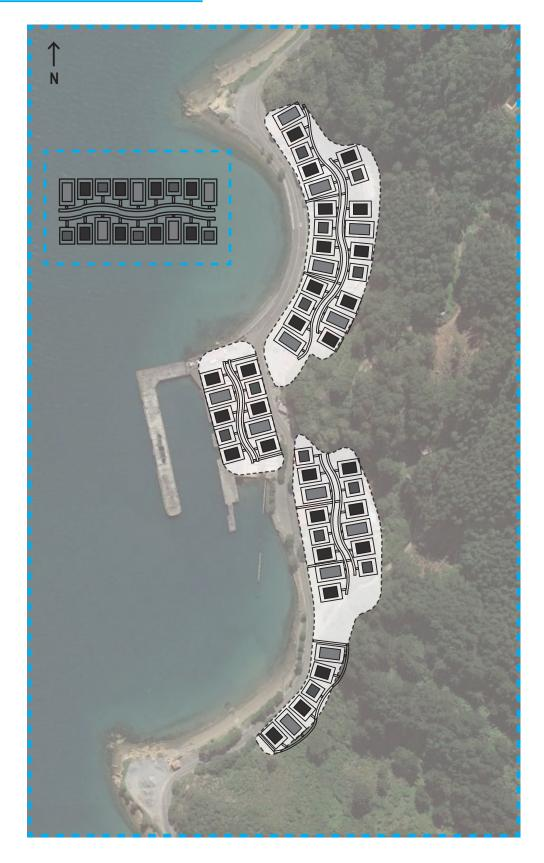
The linear jetty option obstructed the views of the water from the front row of dwellings, whilst the wave jetty option seemed to make the space between the two rows of dwellings appear smaller and confined. A hybrid of the two was established and solved both of those issues. This jetty design works more cohesively with the dwellings alignment, whilst remaining unobstructive from the first row of dwellings and provides for a larger space between the two rows of dwellings.
