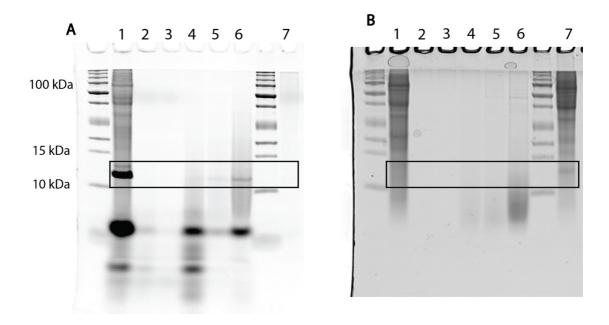
Figure 5-5 DEAE step gradient column separation of MO<sub>F</sub> sample
