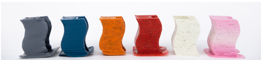
Figure 25: Upcycled filament and 3D test print collection
