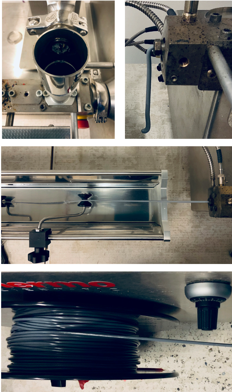
Figure 14: HDPE filament extrusion and spooling process
