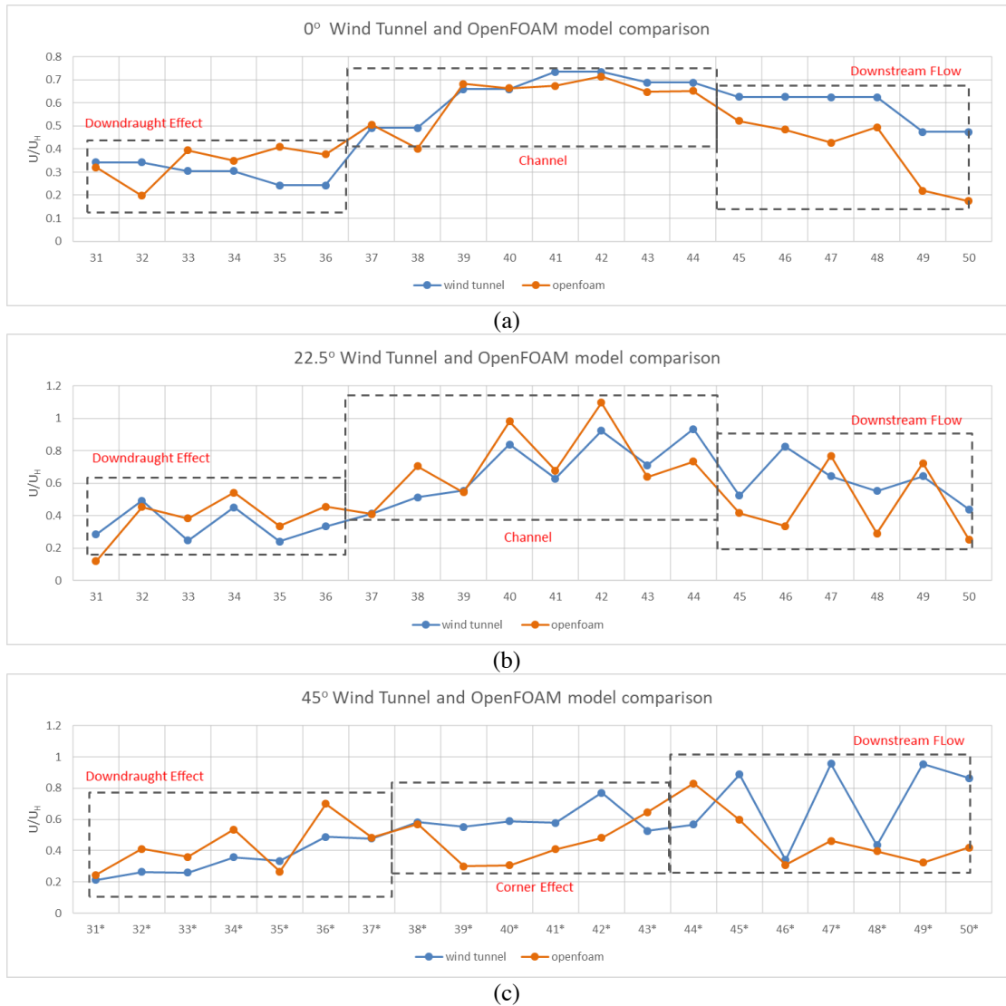
Figure 33: Comparison of wind speed ratio predictions around the central block
