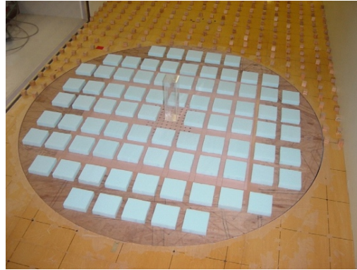
Figure 15: Model of AIJ wind tunnel experiment (Tominaga & Mochida, 2016)
