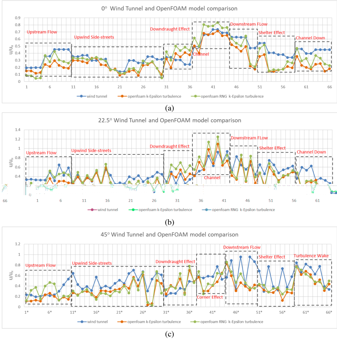
Figure 31: Comparison of wind speed ratios for different turbulence models
