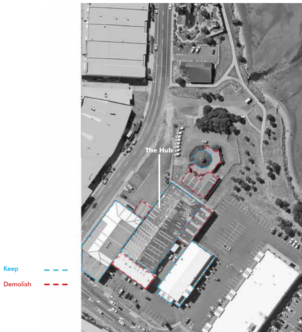
Fig 6.39. Site plan showing buildings to be demolished.
