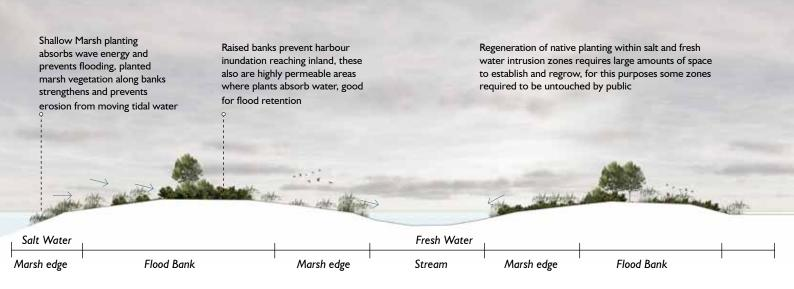
STREAM STRUCTURE. Section B. Public Oriented Zone. 1:150 @ A1
