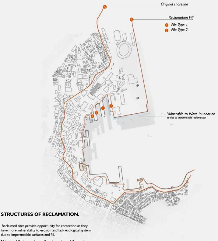
Majority of Ports remain on piles, dimensions of these piles varies between 480-660mm, with 1-2m spreads depending on gravitational loads of buildings. There are two main timber wharf structures within Centreport, the remaining site is Fill. (See Fig.3.16.)
