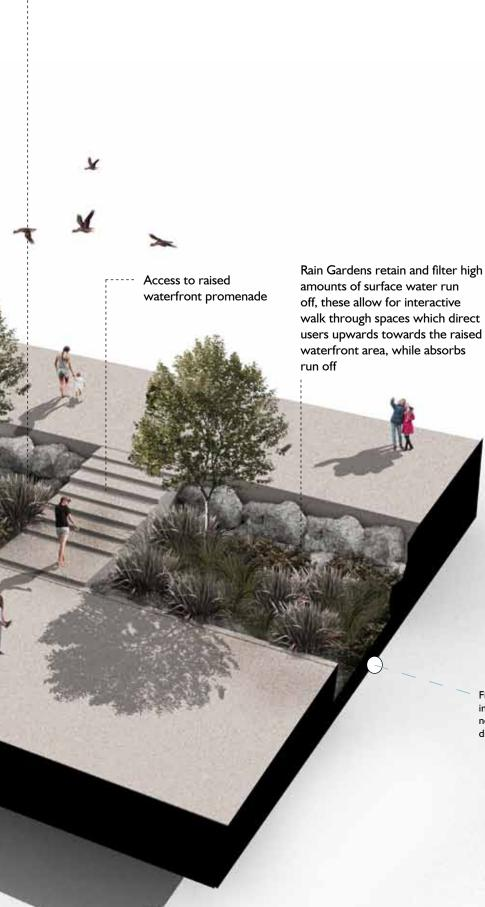
Filtered Rain Water filters into perforated SW pipe network again for later discharge into harbour
