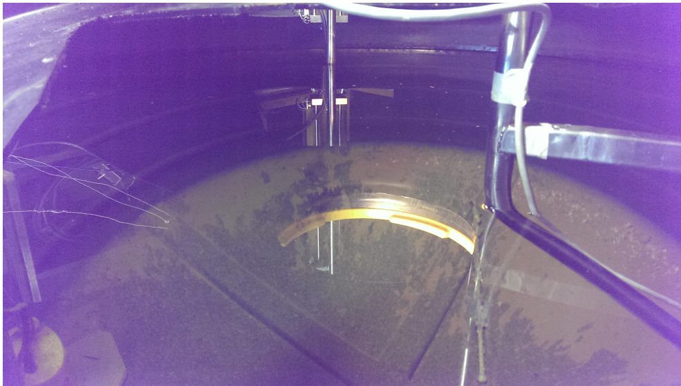
Figure 5.3: Internals of the water tank, showing the hydrophone receiving pulses.
