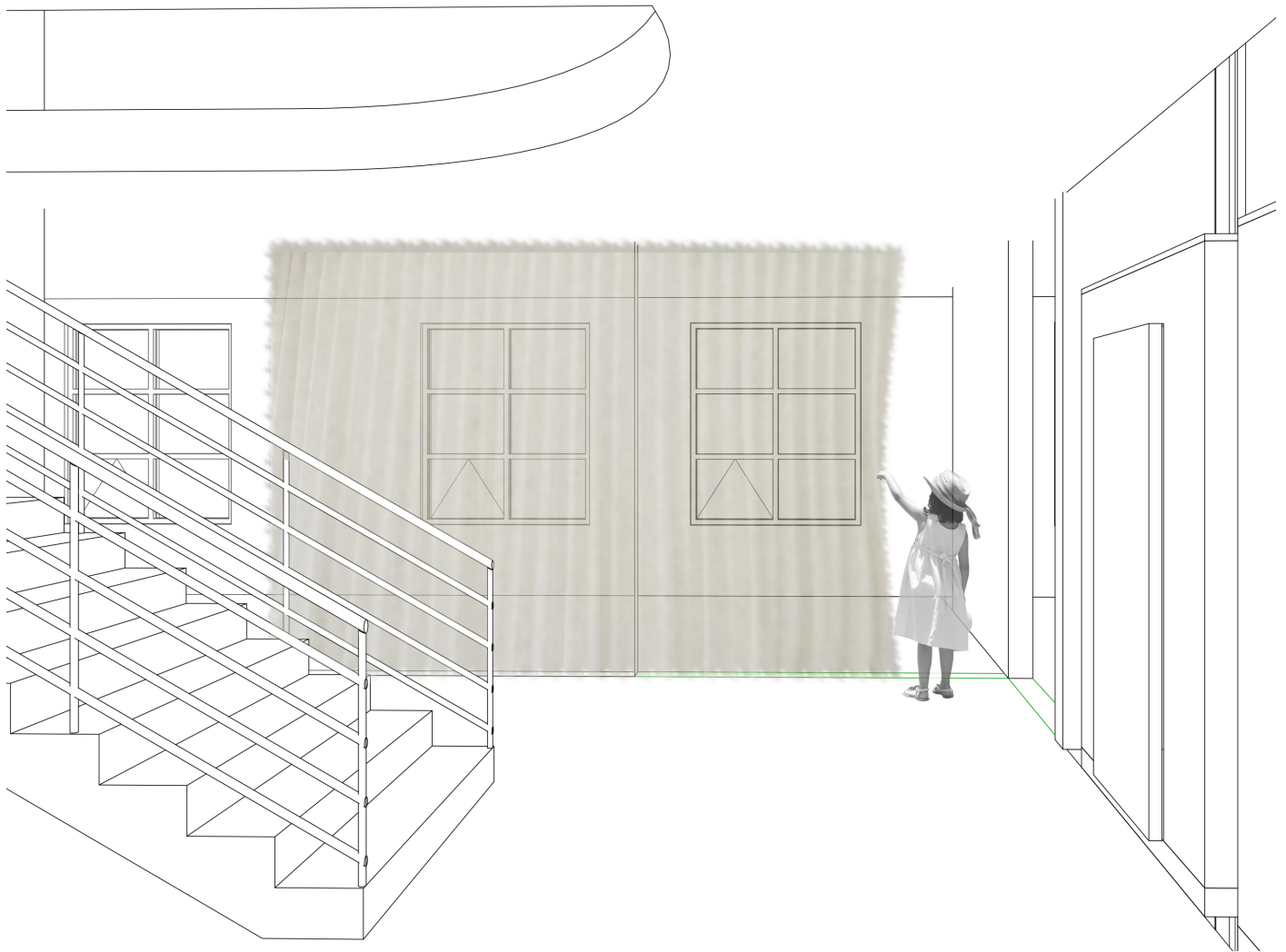
Figure 5.10 View of ground floor exploring partition curtains. This allows spaces to be sectioned off if the space needs to be used for meetings or functions.
