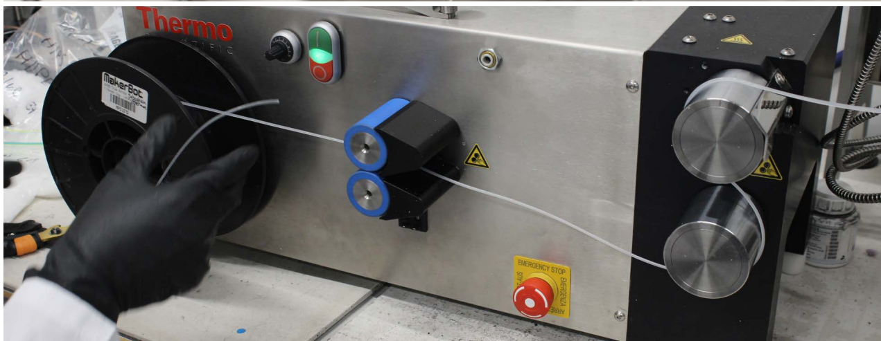
Figure 36: Spooling the Filament
