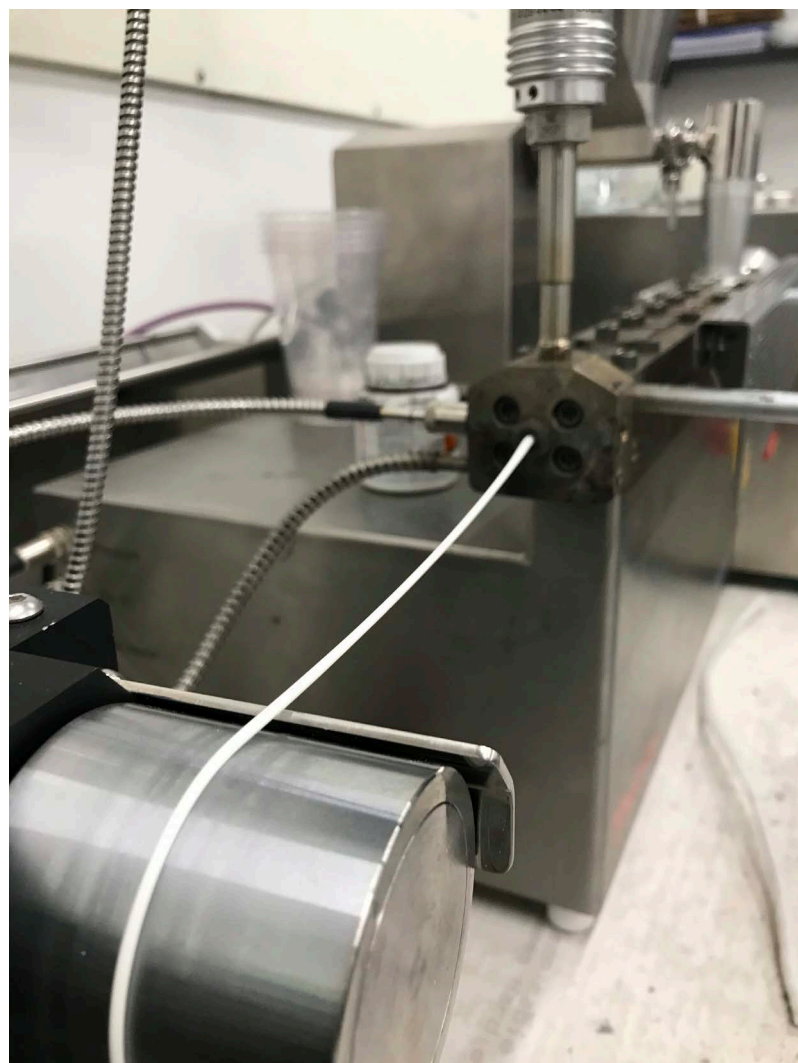
Figure 46: Filament extruding out
