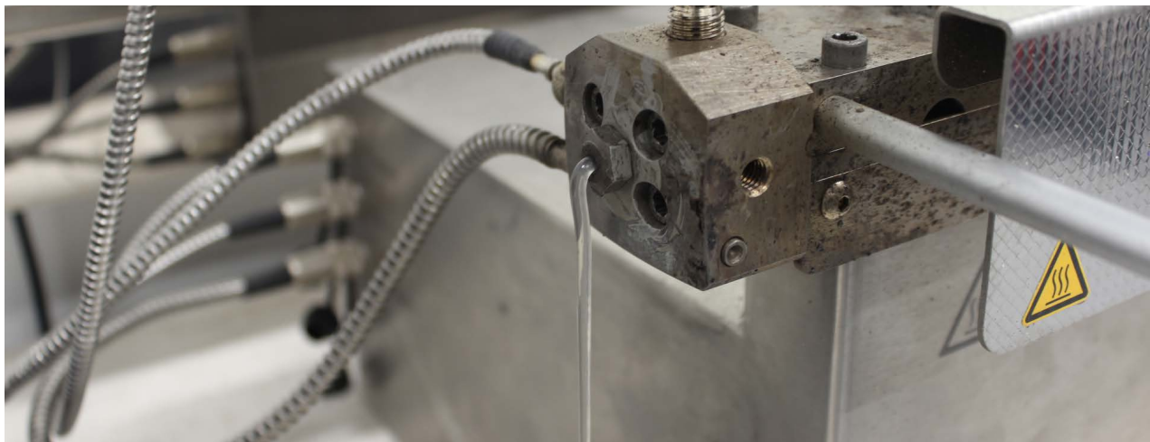
Figure 35: Recycled Plastic Extruding
