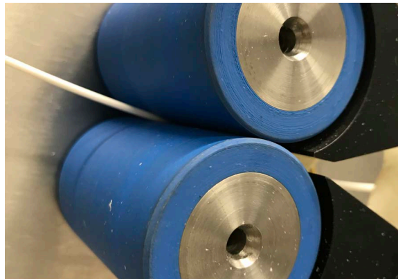
Figure 44: Flattening the filament
