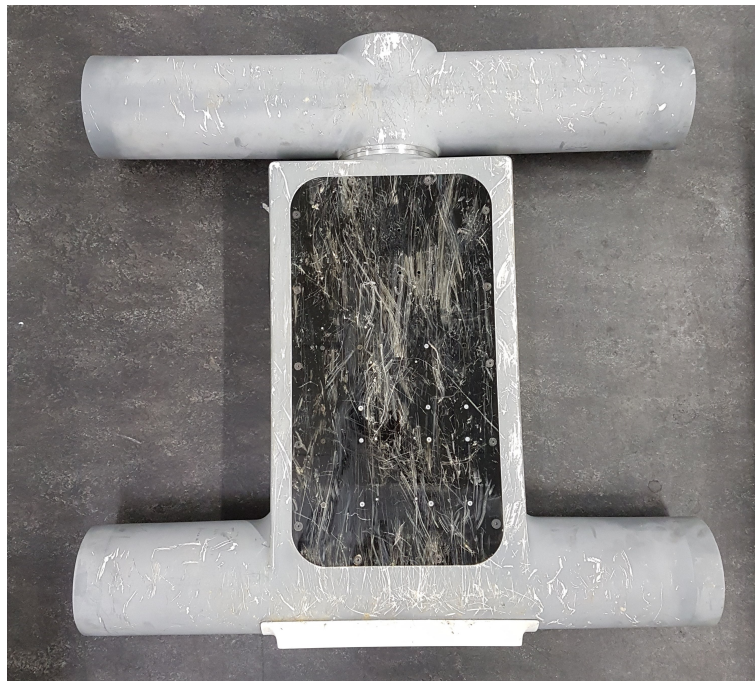
Figure 9.5: The scrapes on the bottom of the HADES chassis from the locomotion tests.
