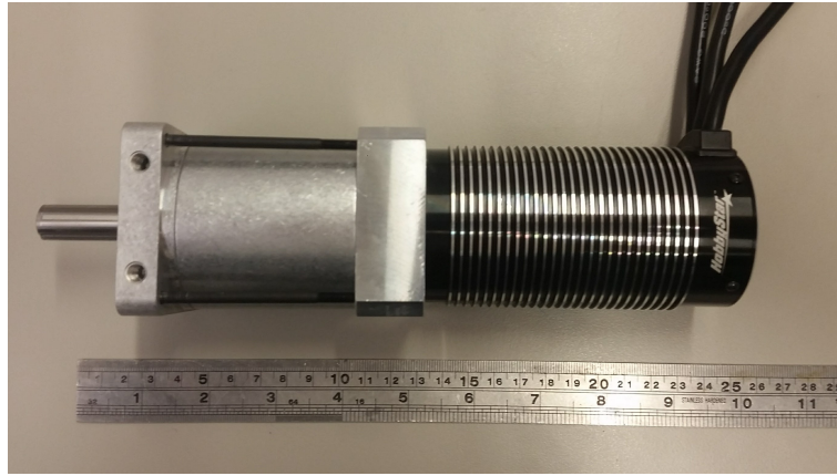
Figure 4.5: The Hobbystar 56112 brushless motor and the Banebots P80 64:1 gear connected together with a bespoke mounting block.
