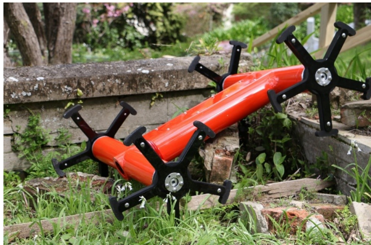
Figure 2.6: HADES revision one climbing over an obstacle.
