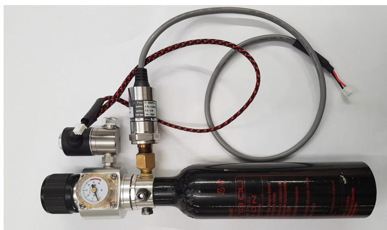
Figure 3.19: The internal tank and regulation system for the positive pressure gas system.
