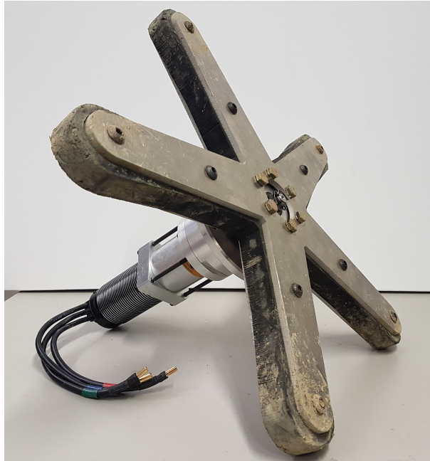
Figure 4.12: The complete locomotion system when it is not mounted inside HADES.
