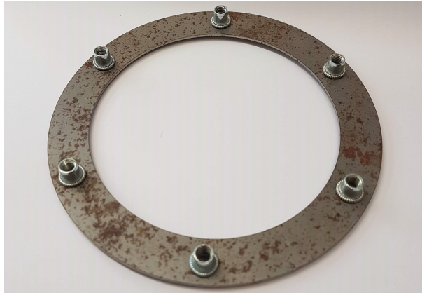
Figure 3.5: The steel insert used for retaining the mounting bolts for the motor and rear arm pivot sub-assemblies.
