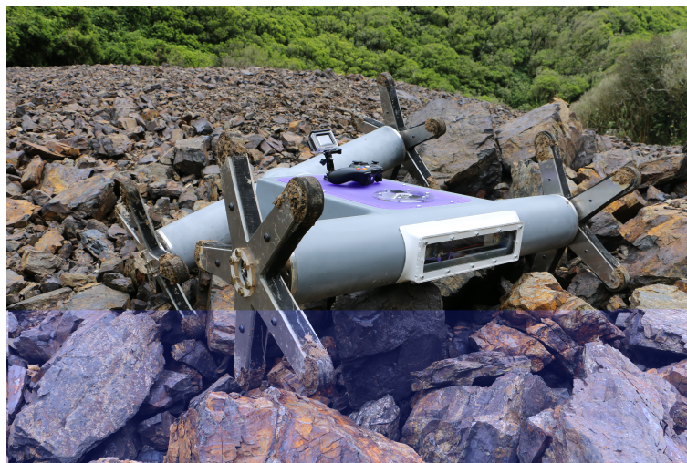
Figure 9.3: HADES travelling over a large bolder field with the two front Whegs not in contact with the ground.
