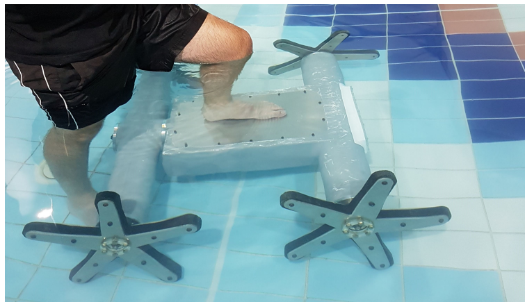
Figure 9.10: HADES being held underwater for the submersion testing of the IP68 standard.
