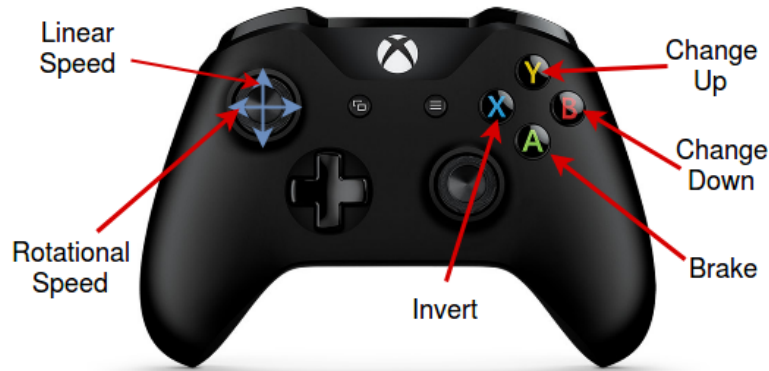
Figure 7.5: The mapping of the different control interfaces to each locomotion control.
