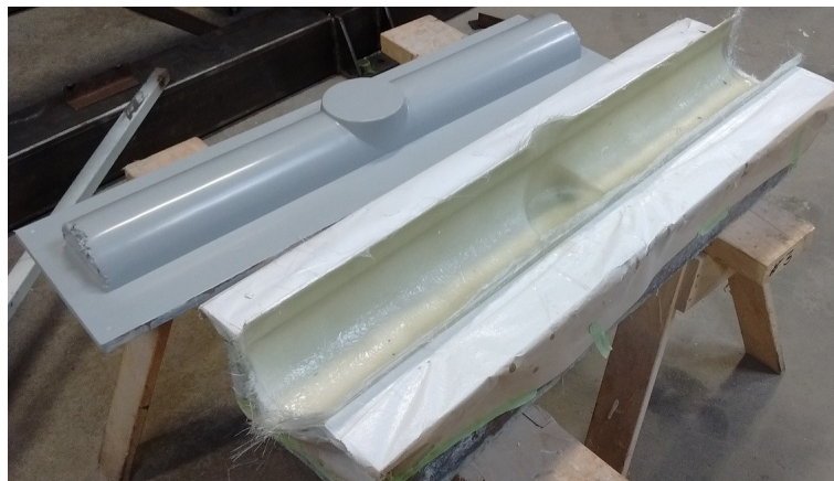
Figure 3.13: The mould plug and mould with a fibreglass part curing in the mould, the indexing tab can be seen on the far side of the moulded part.
