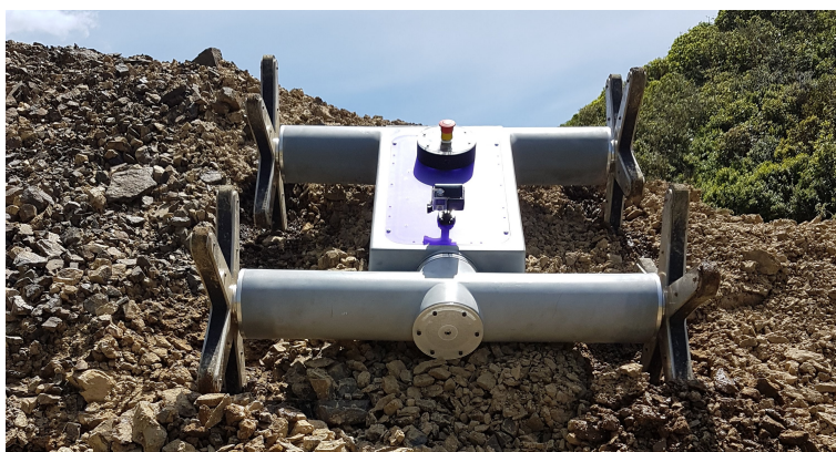
Figure 9.2: HADES bottomed out when travelling up a loose gravel slope due to the Whegs digging into the gravel.
