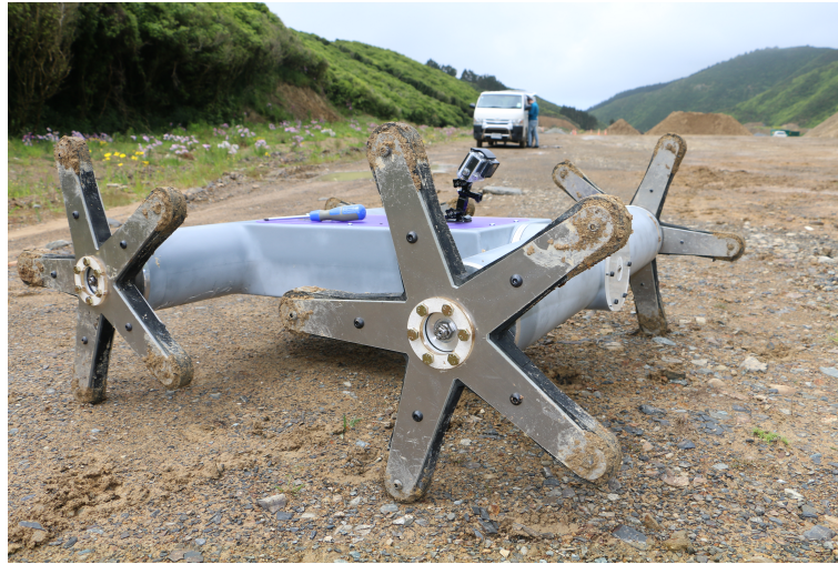
Figure 3.4: The HADES chassis with all the sub-systems and internal components installed.
