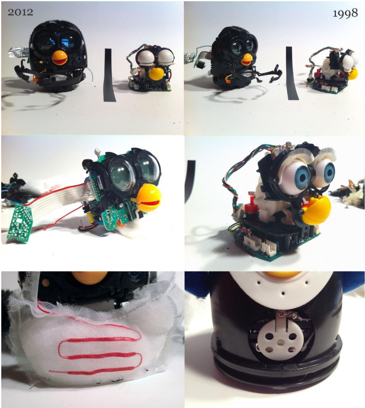
Appendix A. Figure 4 Author. (2012). Comparison details from the 1998 and 2012 Furby dissection.
