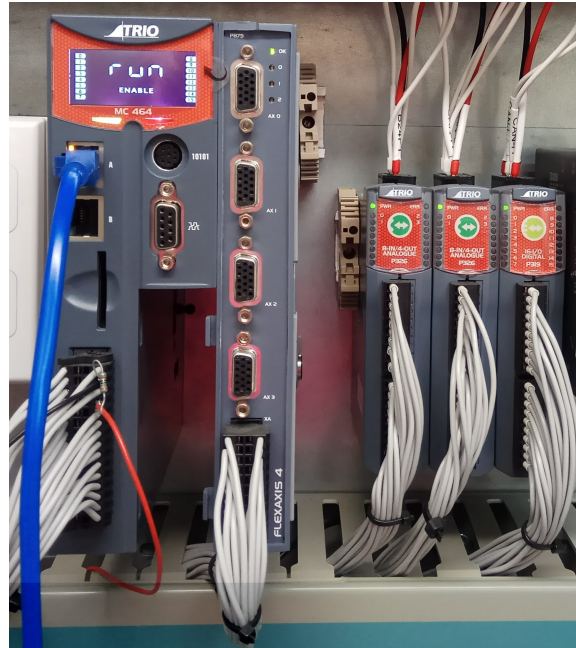
Figure 4.6: TRIO Motion controller MC464 with two analog modules P326 and a digital module P319 in the low voltage cabinet of the ss-CAES prototype.
