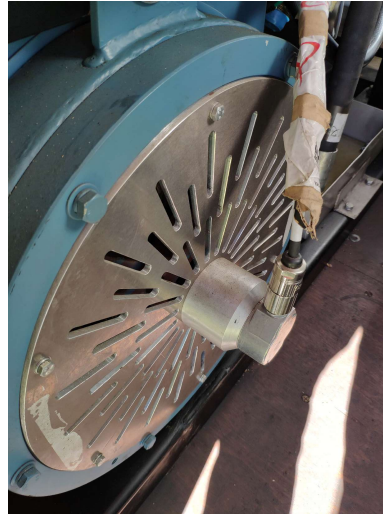
Figure 4.13: SICK DFS60 incremental encoder utilised for measuring the dynamics of the electro-hydraulic drivetrain.
