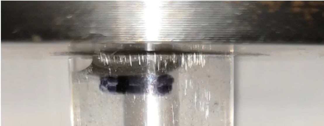
Figure 5.13: The negative field gradient in the top of the enclosed magnetic cell results in fibers collecting in the meniscus of the fluid, which is the opposite of the desired outcome.
