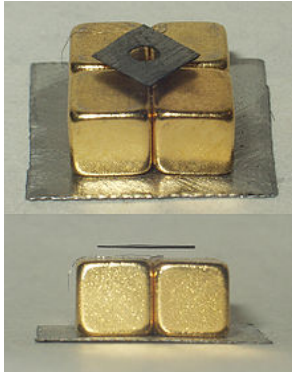
Figure 2.1: Materials with a large diamagnetic constant levitate above strong magnets due to the repulsion force. Pyrolytic carbon is a material with one of the highest diamagnetic constants at room temperature. The magnets illustrated here are 1 cm cubes.
