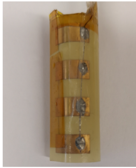
(a) 3D model of the electrode plates. (b) Photograph of the quadrant electrodes
