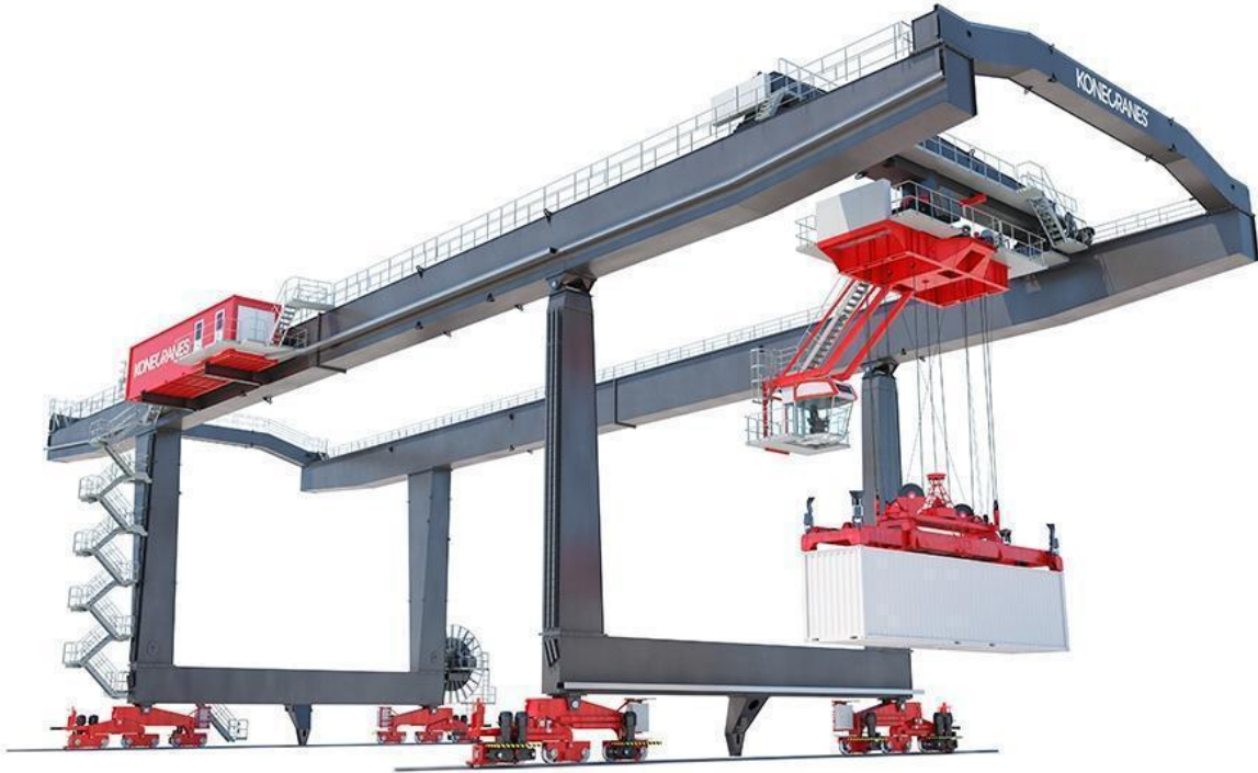
Figure 14 - Overhead rail-mounted gantry crane (Boxporter RMG, retrieved 20 February 2019)
