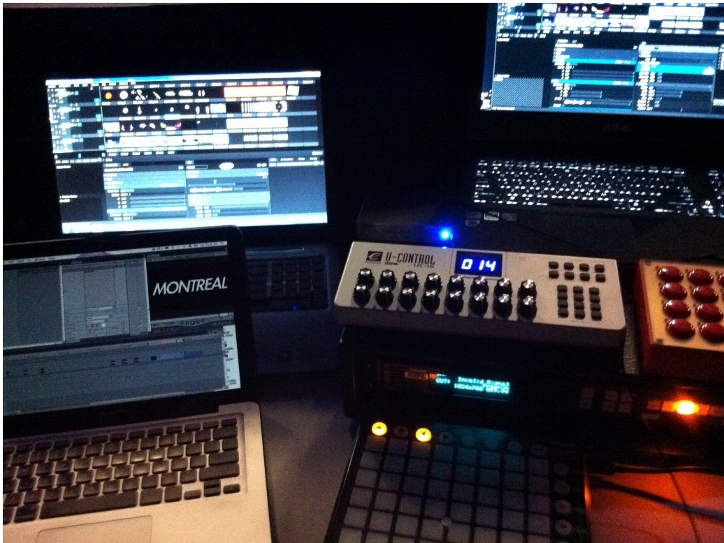
Figure 2.8: VJ setup featuring two PC's running Resolume (top-left, top-right), a MacBook running video editing and patching software for supplemental content (bottom-left), and numerous MIDI controllers (bottom-right) [63].
