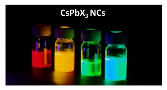
Figure 1.8: A photograph of  $CsPbX_3$  NCs under UV lamp at 365 nm excitation. The emission was tuned by changing the size and composition of NCs. These perovskite NCs show the emission through the entire visible spectrum (490-680 nm).
