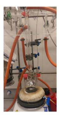
Figure 7.1: A schematic for the synthesis of  $CuInS_2$  NCs with a photograph of the reaction flask during the synthesis.
