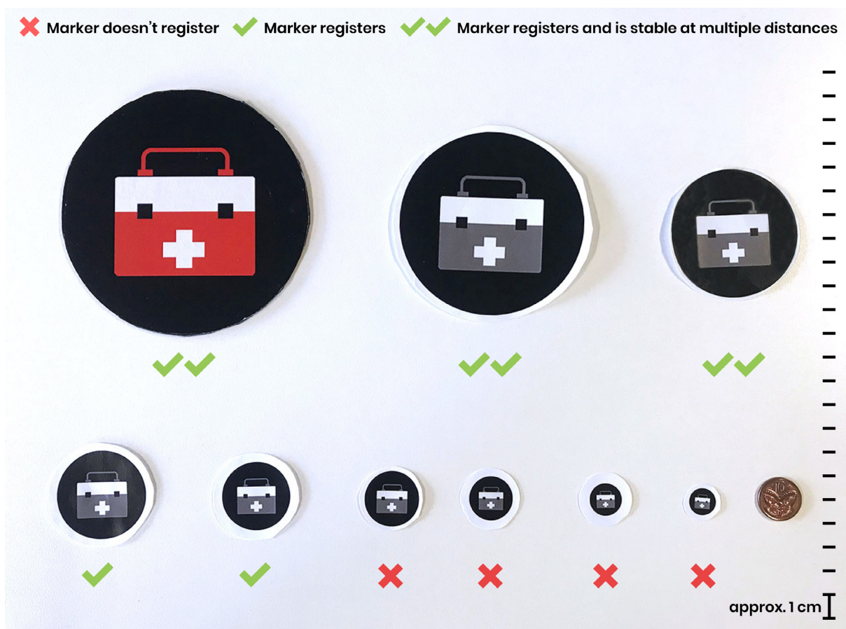
Figure 23. AR marker size testing results with NZ ten cent coin for reference
