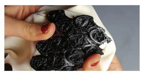
Figure 4.13 3d printed scale structure with increased height to evaluate movement restriction.
