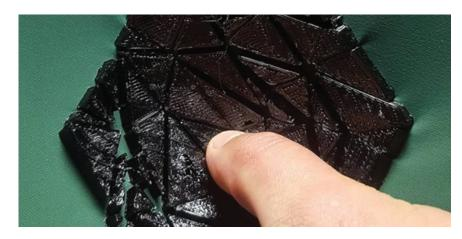
Figure 4.22 Showcasing the locking and expansion of scales when an external force is applied.
