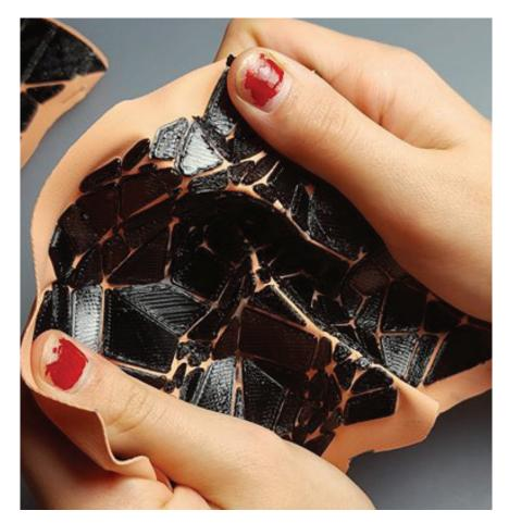
Figure 4.19 Analysing the generated polygon scales in terms of dynamic aesthetic qualities, post 3d print.
