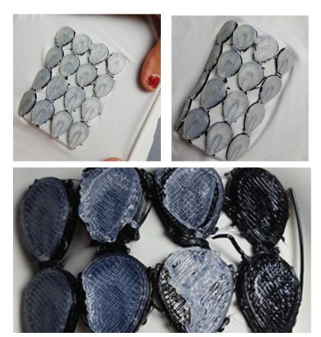
Figure 4.16 Exploring the combination of two 3d printing filaments, to enhance protective capability.
