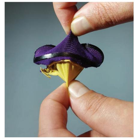
Figure 4.6 Demonstrating the adhesive strength of the layered 3d printed samples.
