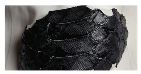
Figure 4.12 Post 3d printing, contouring based on the direction of tension.
