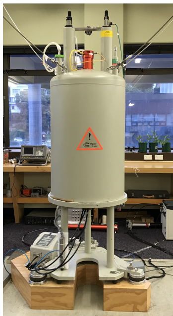
Figure 2.13: Bruker 400 MHz NMR magnet used for this thesis. Console and other peripherals not shown.
