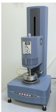
Figure 2.4: TA Instruments AR 2000 stress controlled rheometer used in this thesis. A 60 mm diameter 2^\circ cone and plate shear geometry was used for all testing.
