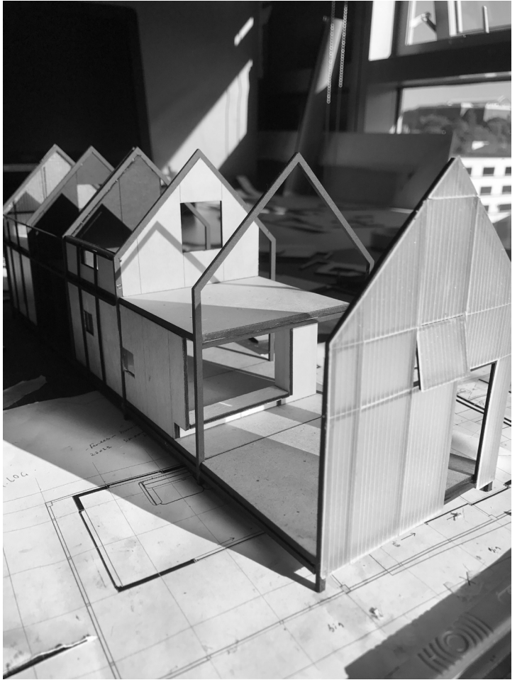
^ Figure 72. / Photographs of the modeling process used to figure out the construction phases.
