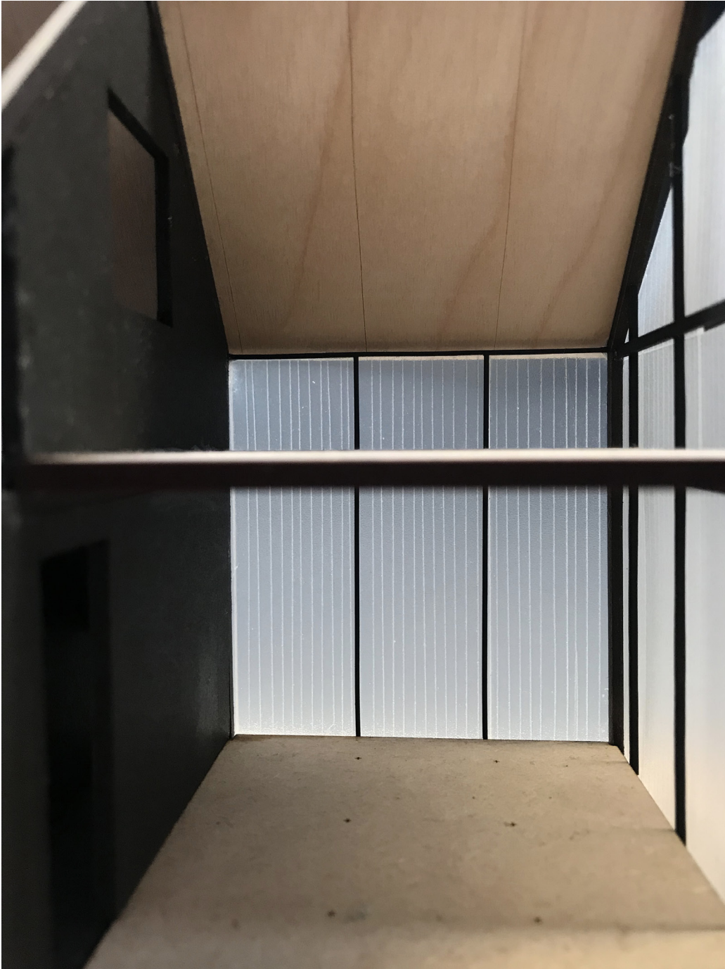
^ Figure 96. / Photograph of physical model interior showing the slack space ready for SIPs to be added into to create an additional room.
