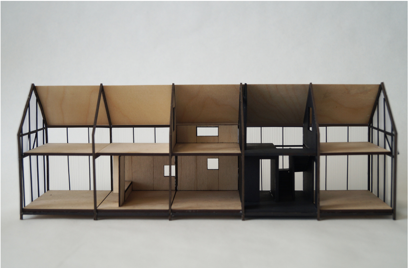
Figure 100. / Photograph of the physical model at stage 1 showing the 5 bays and the slack space either end for expansion at a later stage.
