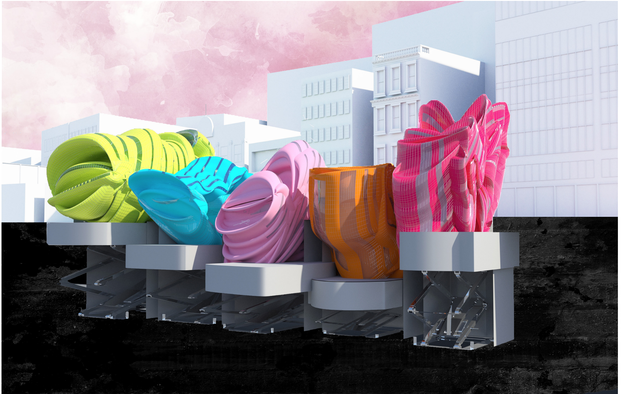
Fig. 5.21 Axonometric section cut showing how buildings move independently via scissor lifts
