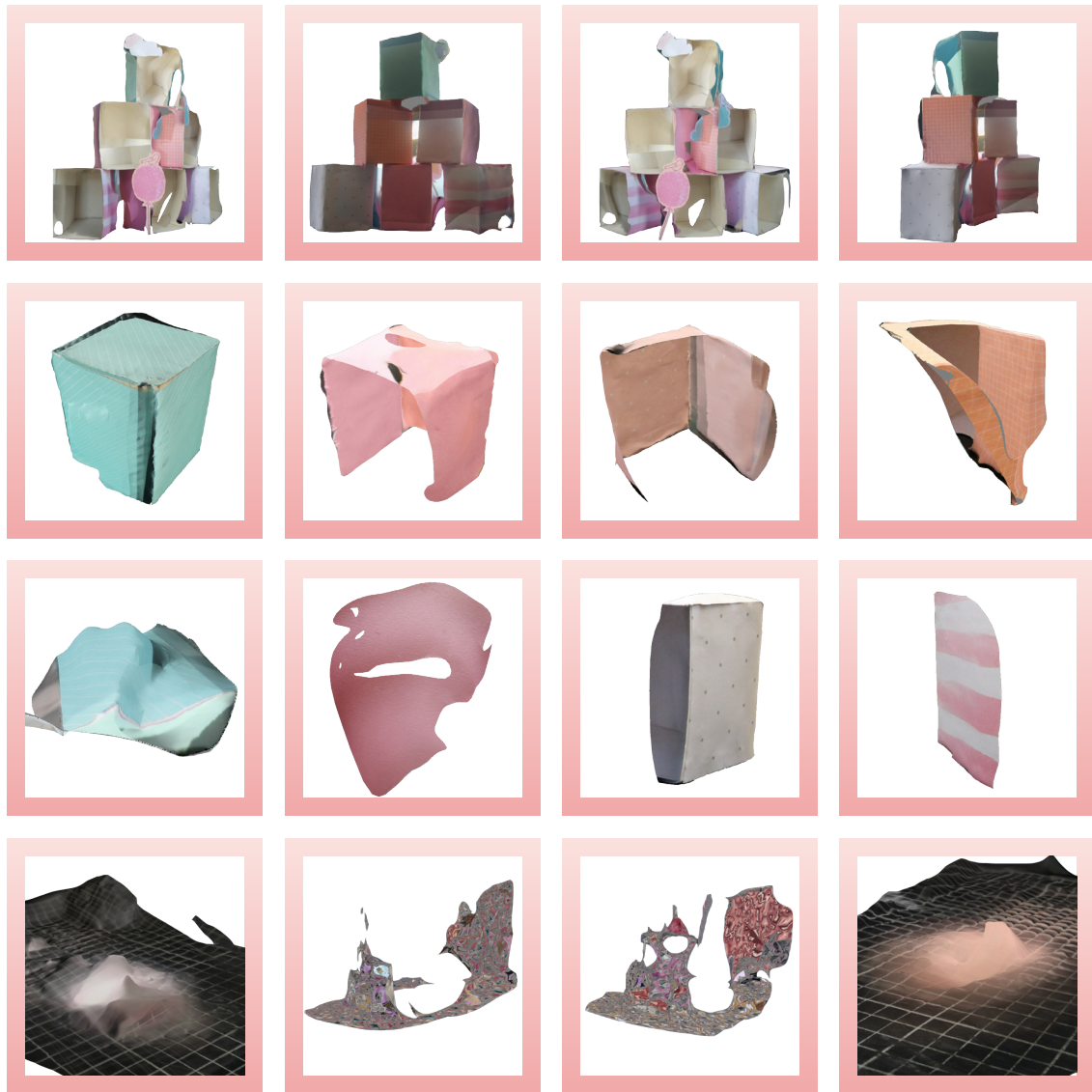
Fig.20. Photogrammetry outcome of exploration 1 featuring many failed attempts. The bottom row show glitches that appeared through some photogrammetry translation of their physical counterpart.
