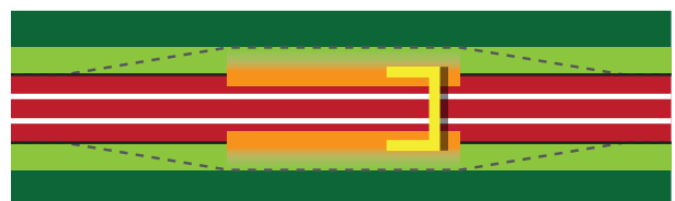
Figure 6.4 Diagrammatic layout of a typical lateral platform train station with overbridge.
