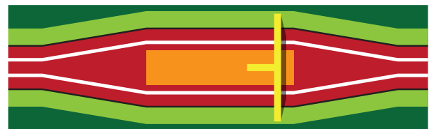
Figure 6.3 Diagrammatic layout of a typical island platform train station with overbridge.
