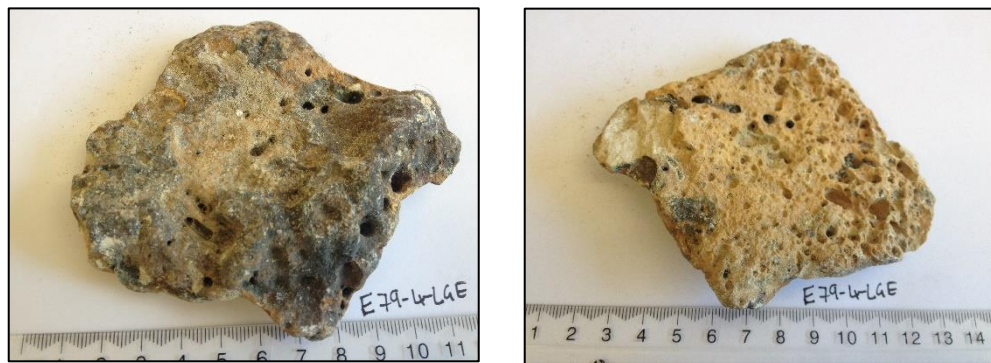
Figure 4-4: Duricrust sample type E79-4-Lge. Left: Top of sample showing vitreous black glaucony mineral. Right: Underside of sample.
