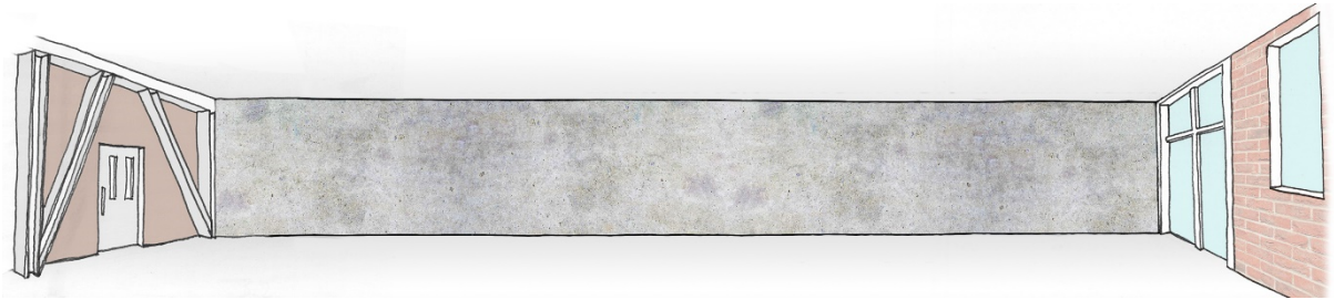
Figure 63. Ornamental exposed shotcreted shear wall running along the entire length of the bar of Building #3
