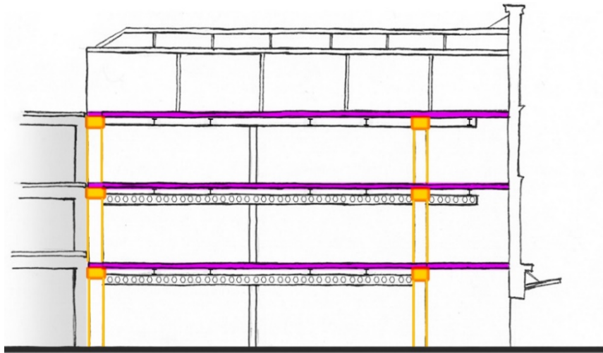
Figure 81. Section of Building #1 showing the moment frames (orange), diaphragms (purple), and castellated beams located at the ground and first-floor
