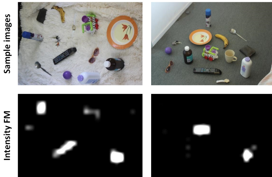
Figure 4.14: Sample images showing intensity variation due to background contrast variation.
