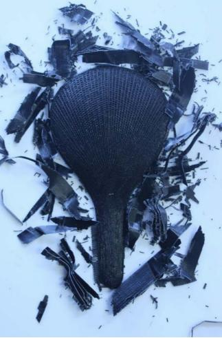
Figure 145(c) FDM Print Oriented Facing Down
