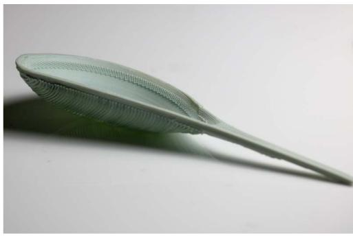
With the measuring spoons requisites of water tightness and marking volume, a layer based approach was adopted. Through Designed Deposition, three-dimensional layering created a watertight structure, and change in patterning was used as volumetric markers.
