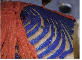
Figure 12. Robotics-enabled stress line additive manufacturing, (Tam, Coleman, Fine, & Mueller, 2016)
