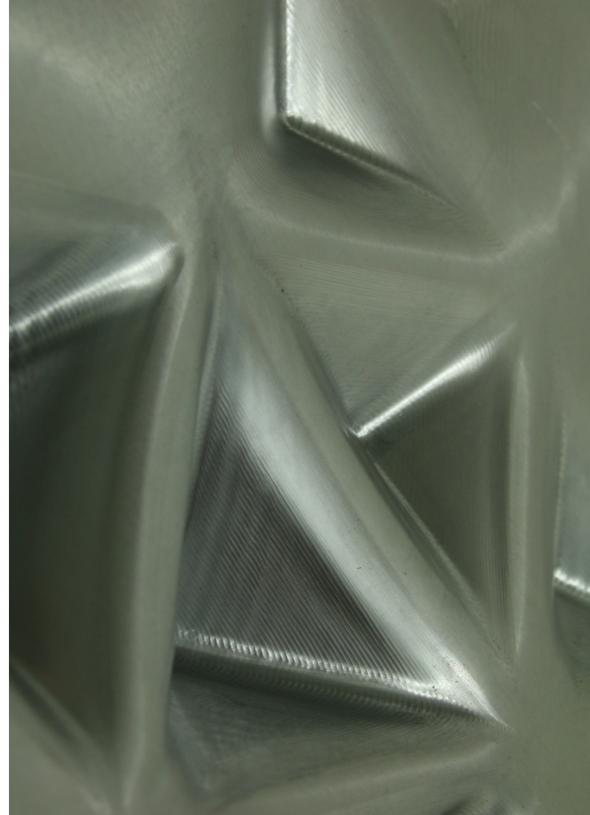
Figure. 44: Distinct forming indentation visible due to corrected incremental step of the forming path (1.2mm increment)
