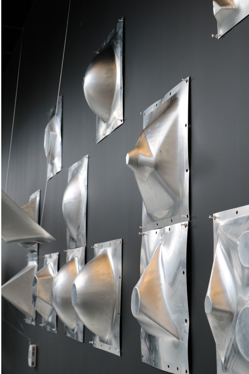
Figure. 18: Panel exhibition: Displaying Phase One incremental forming material exploration
