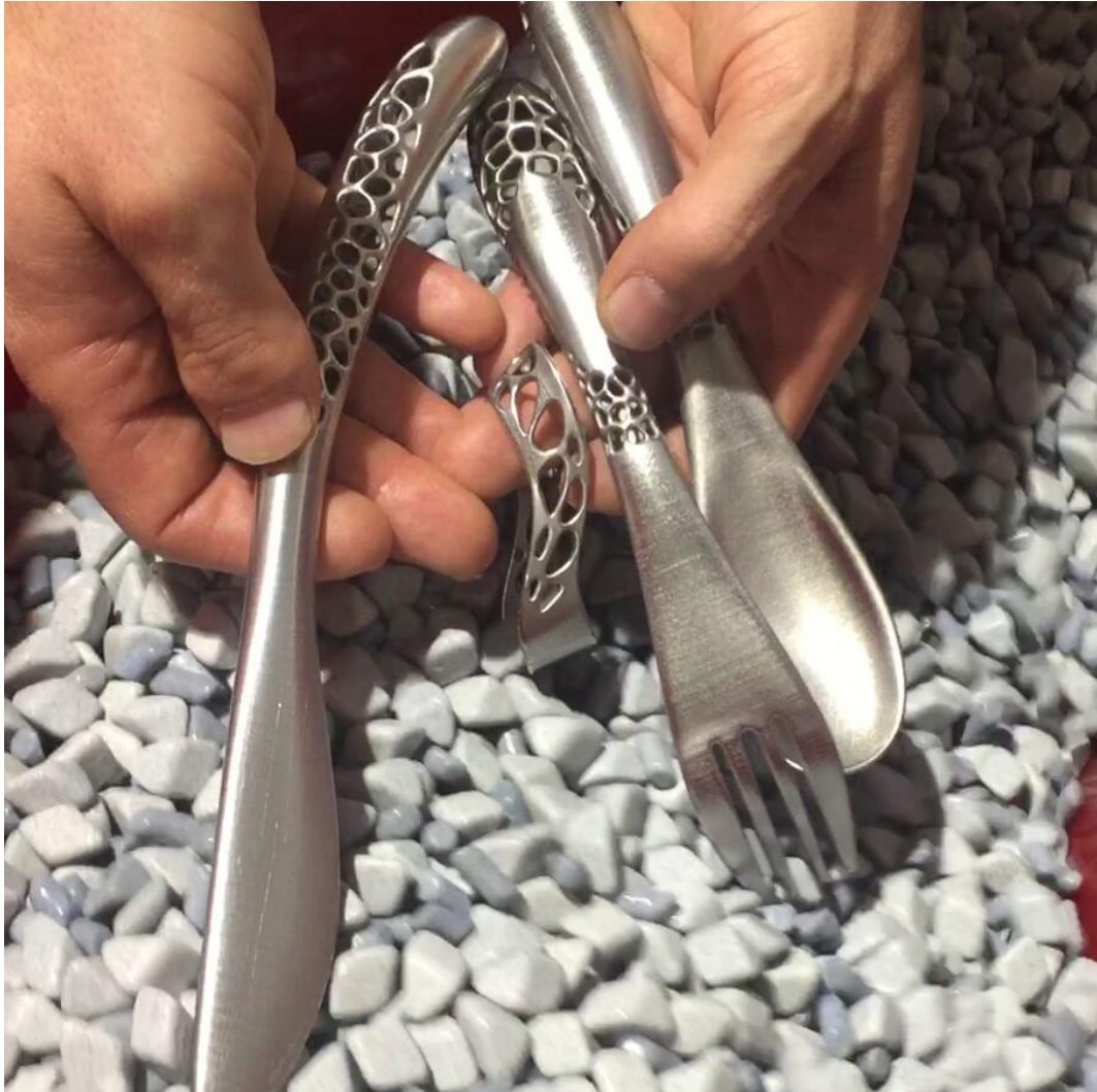
Figure 4.15 3D metal print and polished cutlery.
