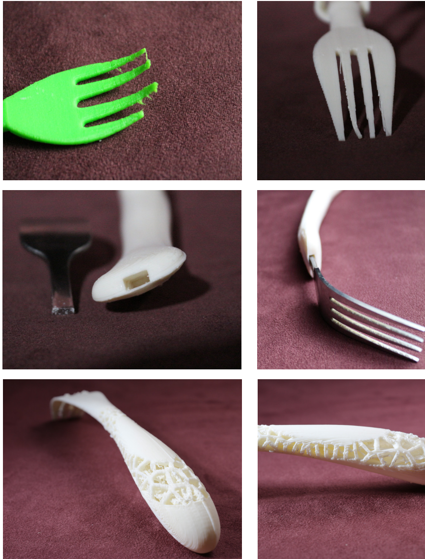
Figure 4.13 Failed front tine of fork (up), combined fork(middle), 3D print meshed fork (bottom)
