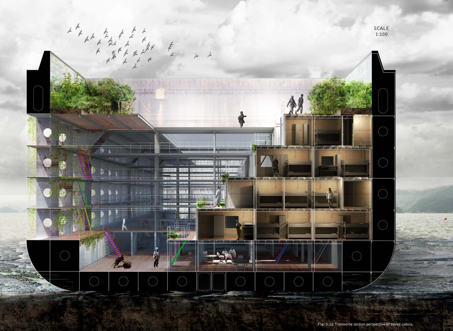
Reconstituted columns and beams are cut from bracing and stiffening members of other ships. These form a latticework that is covered with recycled timber and steel sheets to create new walls and floors. Diffused light reaches here during the day, at night this space is lit artificially, powered by diesel generators retained in the ships engine room. As people pass through here on their way to work, or their cabins, they have the opportunity to socialise with their peers.
