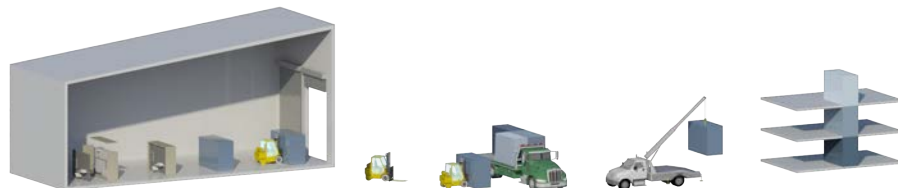
Figure 5.31. Servicebox delivery and installation process
