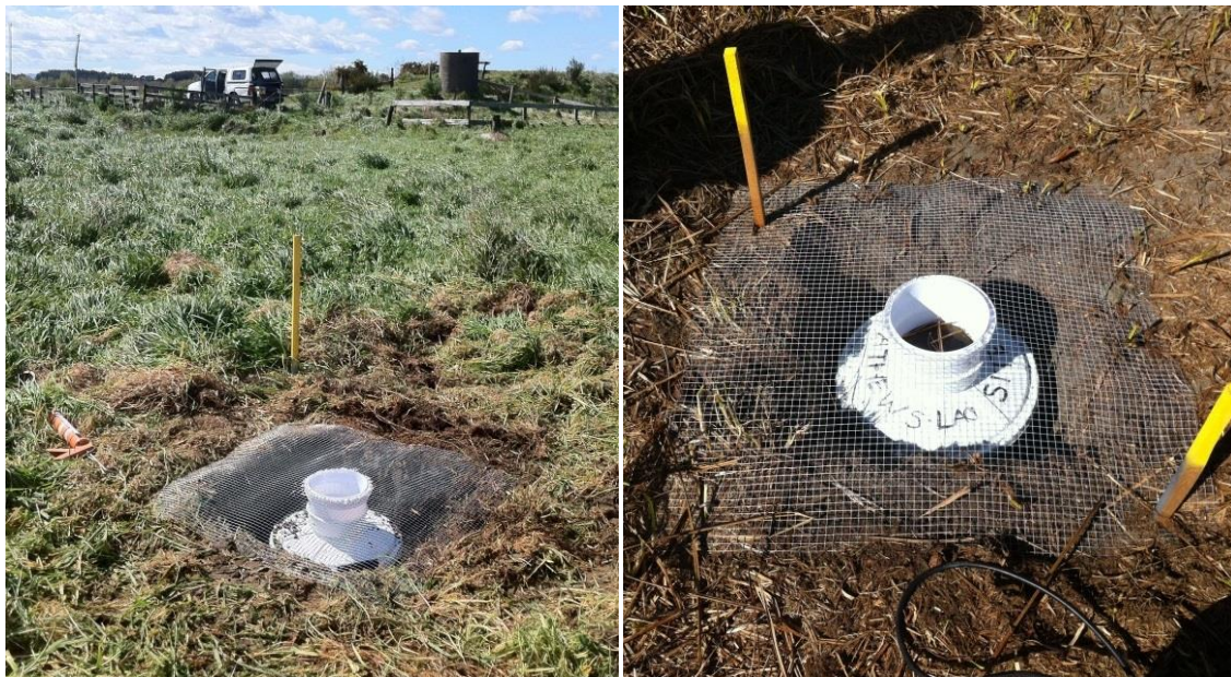
Figure 5.9: Installation of two pit gauges, the control gauge and the Lake Wairarapa gauge (prior to the inclusion of the solar reflection boards)
