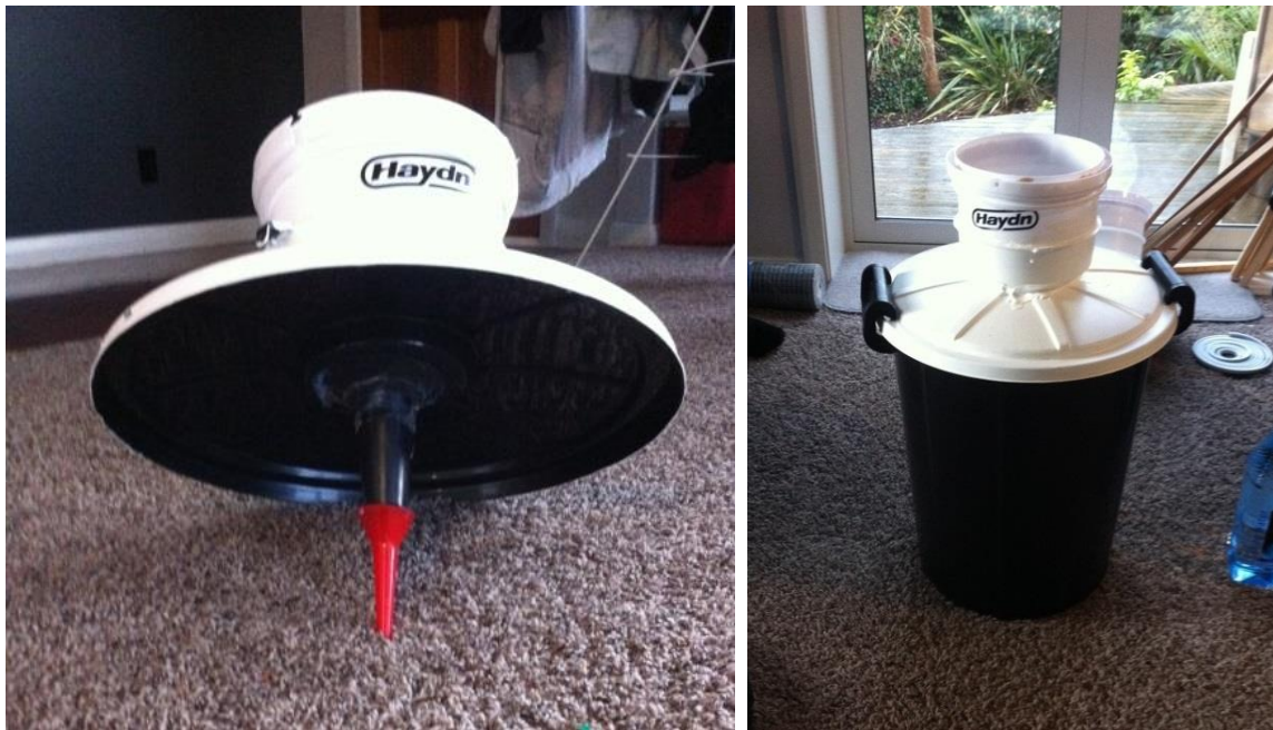
Figure 5.6: Constructed pit gauges for use in the measurement of wind driven rain on the eastern shore of Lake Wairarapa
