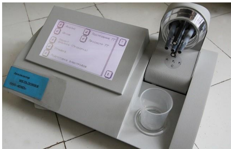
Figure 6: Prototype of an Electrochemical analyser, developed by Olga Mezentseva at Tomsk Polytechnic University.
