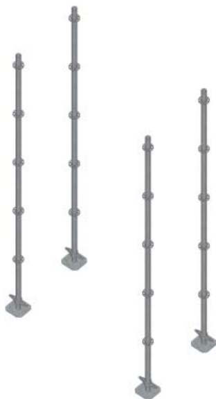
Standard Scaffolding system Each connection point is located at 500mm centres
