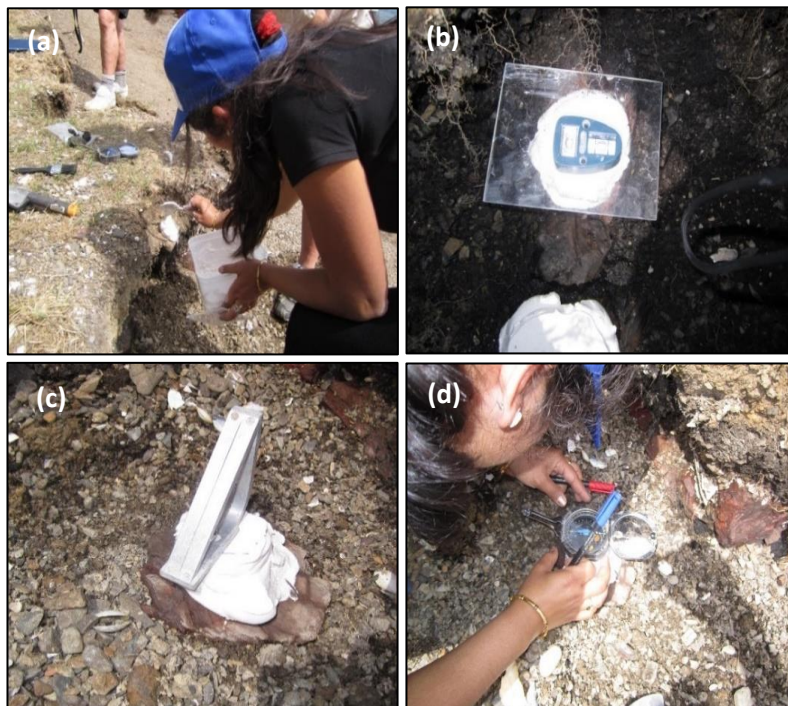
Figure 2.2. Sampling method. (a) Hangi stone covered with plaster of Paris. (b) Levelled poP on top of stone with the help of bubble level and Perspex. (c) Sun compass placed on levelled top for marking sun-direction. (d) Compass needle to mark magnetic north direction.
