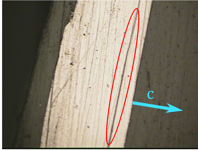
Figure 4.9: Optical microscope image of the cross section of an epoxy potted air-annealed \text{FeSe}_{0.35}\text{Te}_{0.65} single crystal prepared for Raman spectroscopy and SEM analysis. The area marked by the red ellipse highlights a region, where the crystal was split. The light blue arrow indicates the c axis of the crystal structure.
