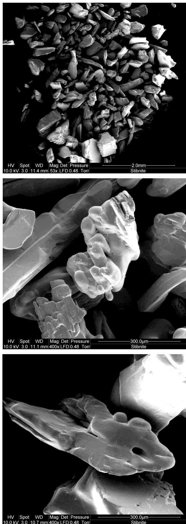
Figure (A.2) SEM images of reacted stibnite from high temperature experiments. Images demonstrate grain-size distribution and embayed surfaces of reacted grains, including preferential dissolution parallel to the c-axis.
