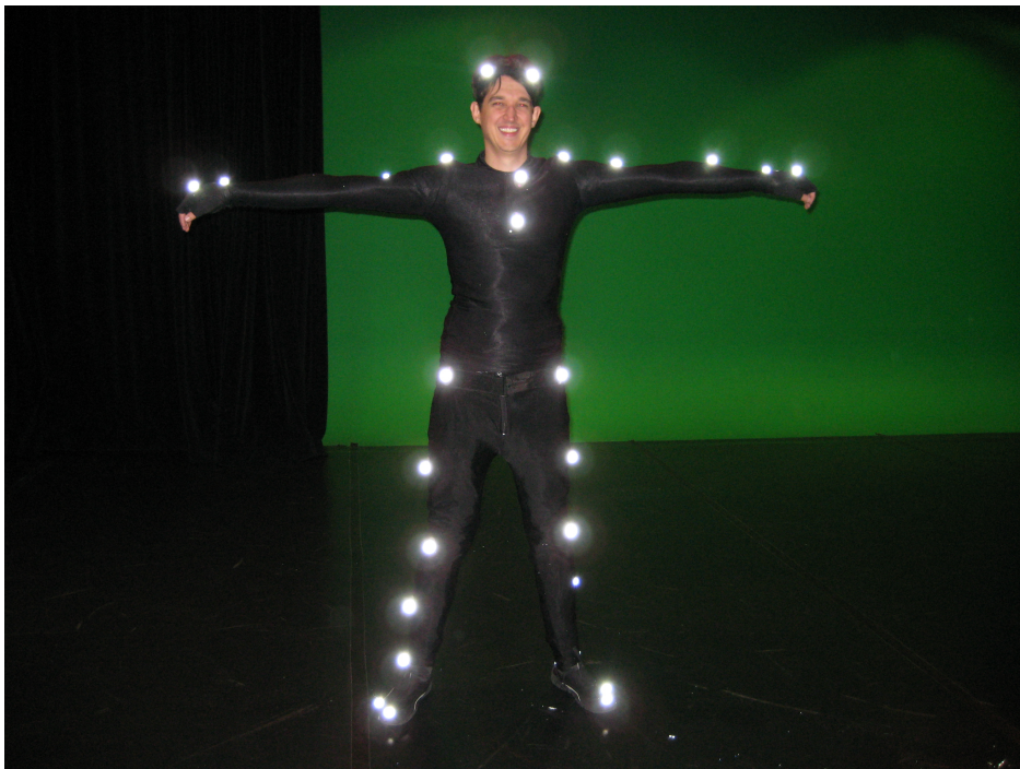
Figure 2.2: Active marker mocap system. Light-emitting markers are tracked by video cameras. Image licensed by creative commons [18].
