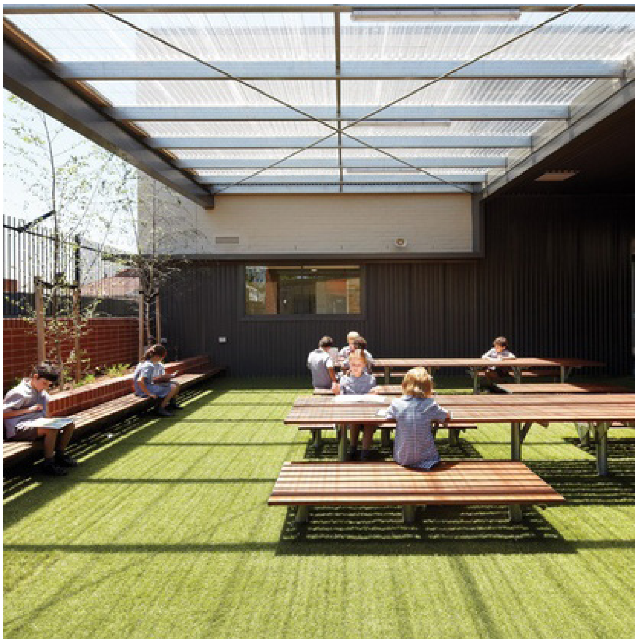
▲ Fig 2.18. Warm shade, the use of transparent shade materials, has potential to shield UVR levels whilst providing for thermal comfort with infrared transmission (Mackay et al., 2014).
