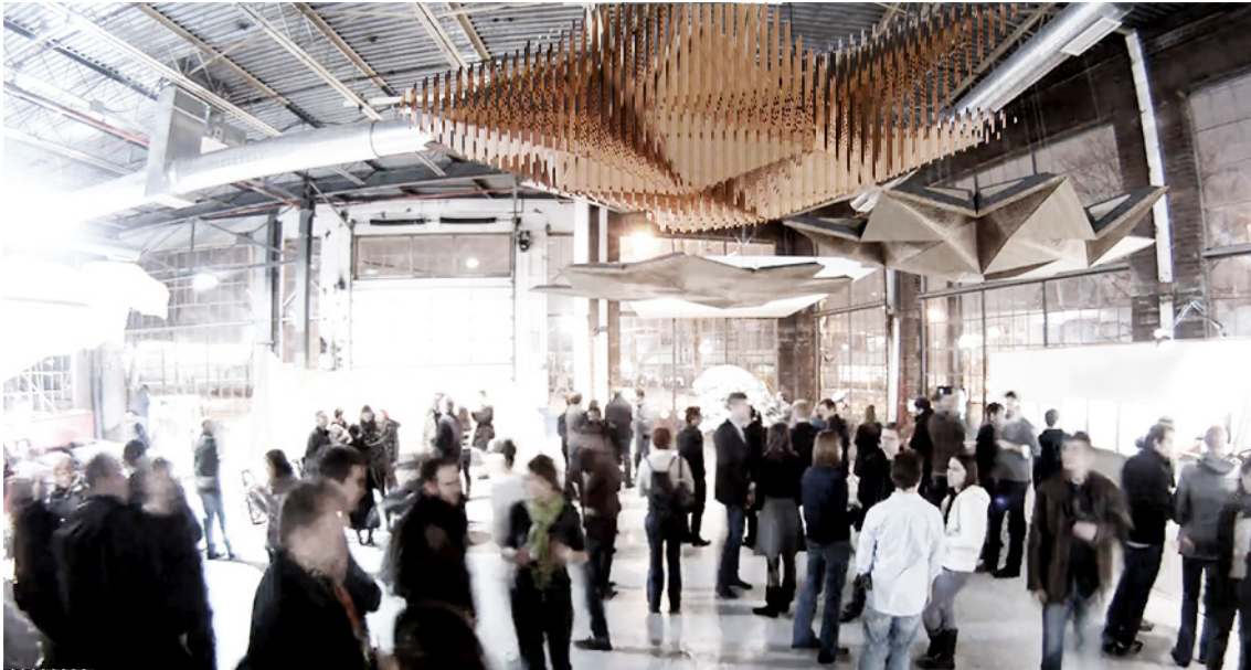
▲ Fig 2.35. Resonant Chamber. Acoustically responsive ceiling panels are activated by microphone and controlled by dual hydraulic actuators on the back of each junction allow acoustic control.
