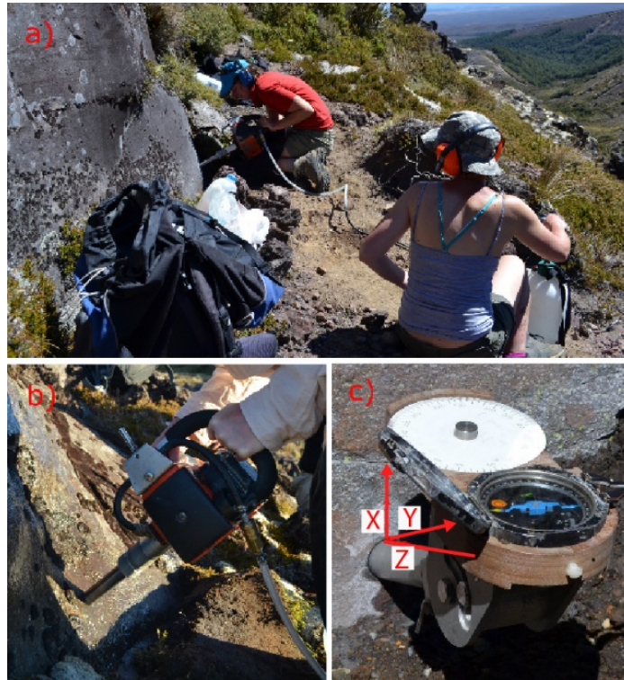
Figure 2-1: Sampling method: a) Author coring an andesitic lava flow on the left and assistant operating pressure sprayer to enable cooling water flow. b) close-up shot drilling. A petrol driven drill with a diamond bit of 2.5 cm diameter is used to core the rock. c) Orienting of a drilled sample prior to removal from the bedrock, the sample coordinate system is indicated in red. Plunge (angle between z and horizontal) and azimuth (angle between magnetic north and y) are measured using an inclinometer, sun- and magnetic compass.
